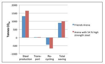
Reduced greenhouse gas emissions for the Friends Arena and a fictive structure with 54 % high strength steel, compared with a structure of conventional steel only.
