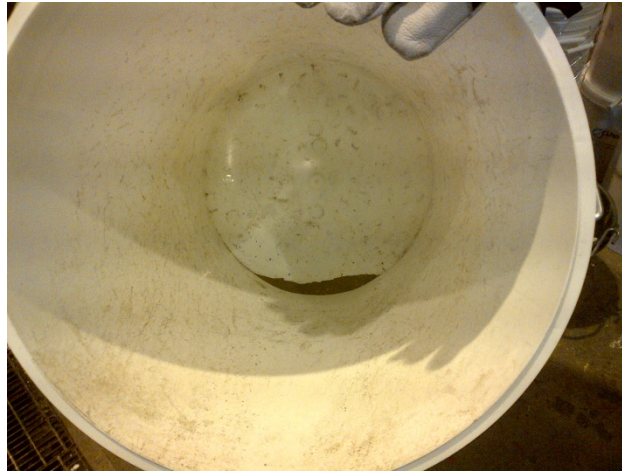
Figure 7. Virtually no fines generated during the long distance transportation of Booster™
