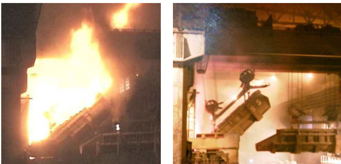
Figure 6: Scrap charging in hot metal, scrap chute without (left) and with cover (right)
