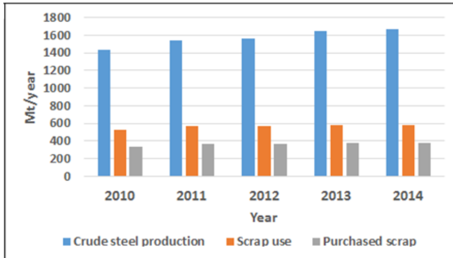
Figure 4. Scrap use for steel production and amount of purchased scrap as well as the total world steel production 2010 – 2015 [12].
