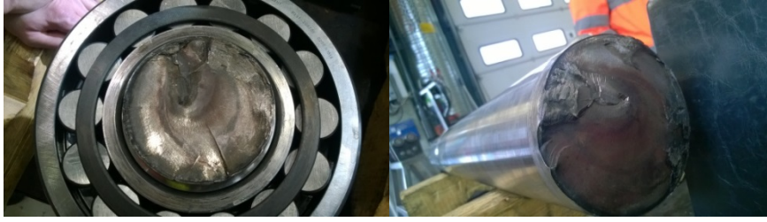
Figure 17. Broken driveshaft of GAD2.
