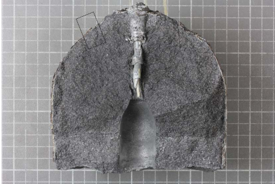
Figure 1 – MgO stopper rod tip after recovery and cutting. The central purging outlet is in the centre of the tip. Black box marks SEM-sample location.
