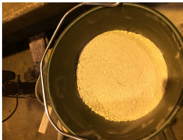
Figure 6. Up to 7% of fines generated during sieving of quicklime
