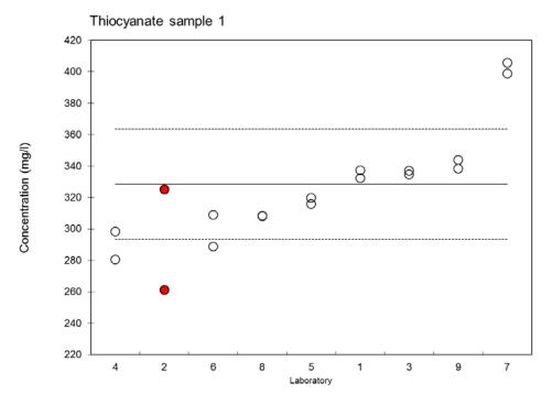
In the graph colored values indicate that the testing machine is a statistical outlier; red – Cochran outlier, blue – Grubbs single outlier, green – Grubbs by pair outliers. Straight line indicate mean value and broken lines  $\pm 1 \sigma$ .
