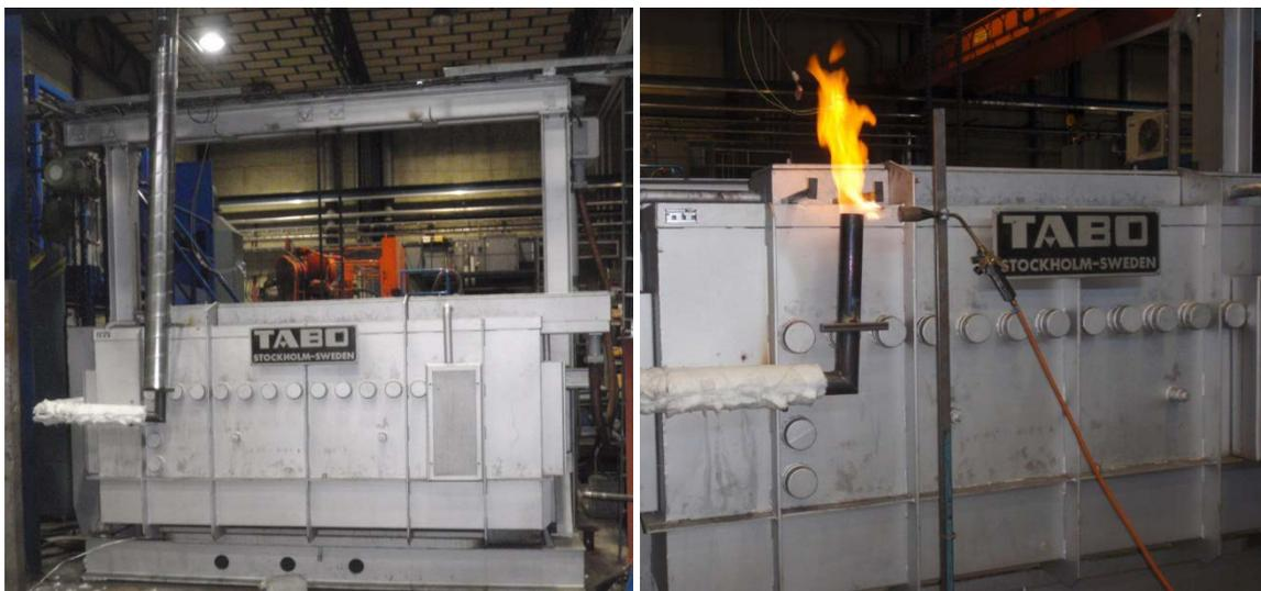
**Figure 9** Exhaust gases directed to off-gas system (left) during warming- and heating period. During reduction period, off-gases from furnace were burned.
