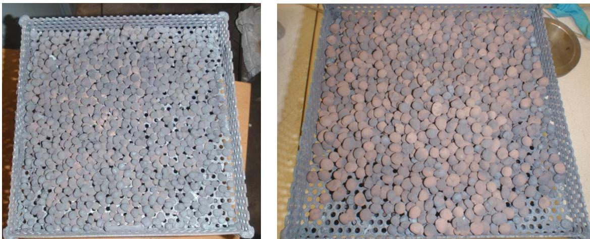
Figure 58 PM1 Pellets after trial 22/4 (left) and 24/4 (right).
