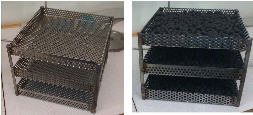
**Figure 13** Construction designed to enable reduction of pellets.
