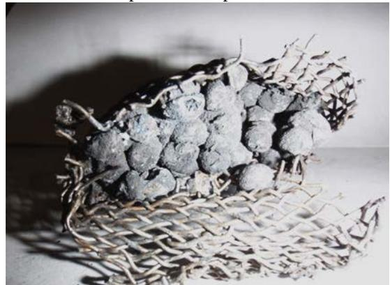
**Figure 87** After excavation; basket L37B4 that was filled with PM1 pre-reduced pellets from trial 22/4.
