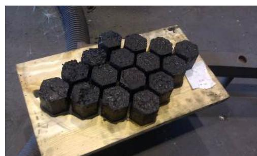
**Figure 4** Pallet of produced lab-scale briquettes.
