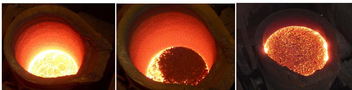
**Figure 52** Heat X1188 before charging (left), after charging bag 1 (middle) and after charging pig iron (right).
