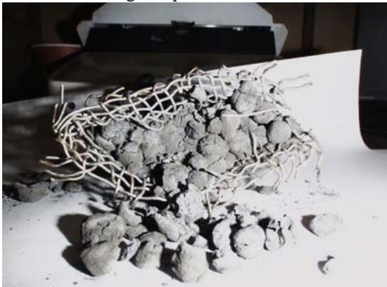
**Figure 86** After excavation: basket L33B7 that was filled with PM1 green pellets.
