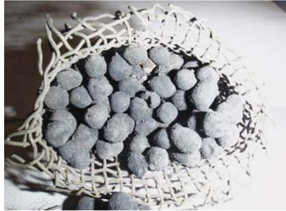
**Figure 85** After excavation; basket L17B3 that was filled with PM1 pre-reduced pellets from trial 22/4.
