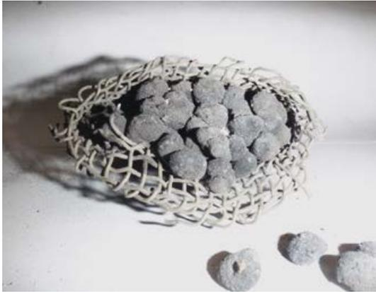
**Figure 84** After excavation: basket L17B1 that was filled with PM1 green pellets.
