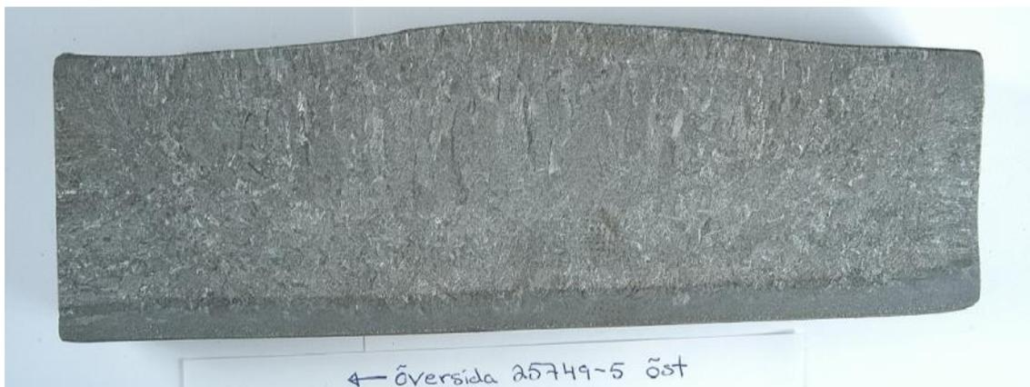
**Figure 93.** Photo of etched east narrow side transverse slab sample (arrow points at upper-loose/north side).
