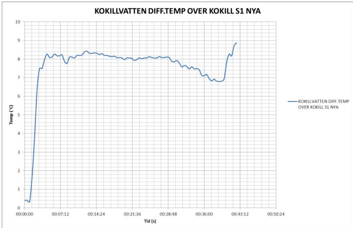
**Figure 56.**  $\Delta T$  of mould water.
