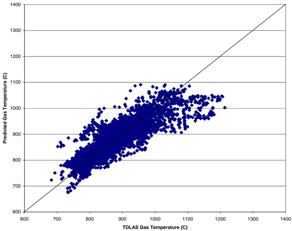
Figure 14. Predicted gas temperatures in furnace 302 versus gas temperatures measured with the TDLAS.
