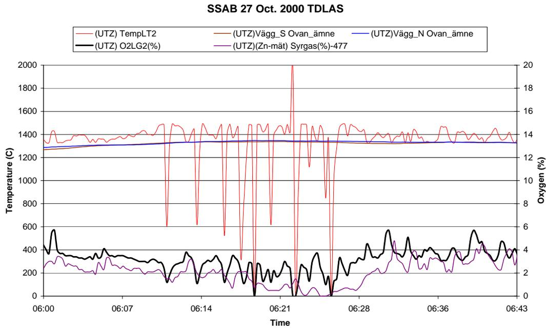
Figure 9. An expanded time scale for of the instability in the simultaneous measurement of the excess oxygen and temperature in the soaking zone of SSAB Furnace 302 at low levels of excess oxygen at 6:20.
