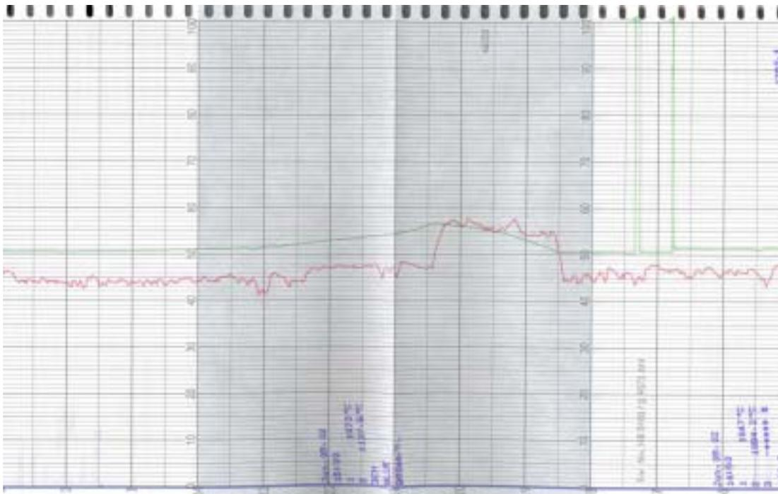
Figure 3. Combustion gas temperatures (wavy red line) compared with the ceiling thermocouple in the lower section of zone 2 with varying burner output from 0 to 100 %.
