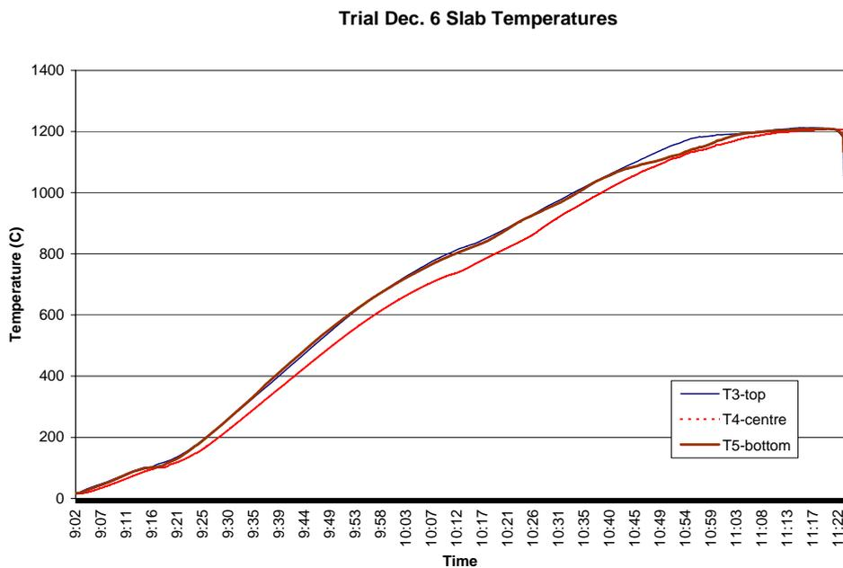
Figure 13. Thermocouple temperatures at position 4 (middle) of the test slab at SSAB, with the top, centre and bottom slab temperatures.
