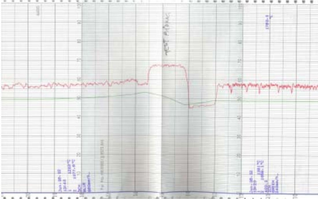
Figure 2. Combustion gas temperatures (wavy red line) compared with the ceiling thermocouple in the upper section of zone 2 with varying burner output from 0 to 100 %.
