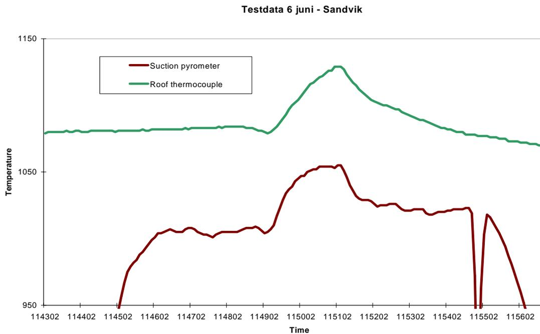
Figure 6. Temperature with the suction pyrometer at the lower position in zone 2.
