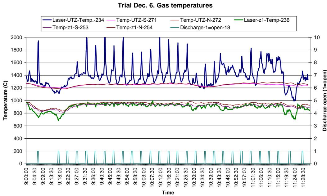
Figure 11. Gas temperatures in zones 1 and 5 during a data logger trial.
