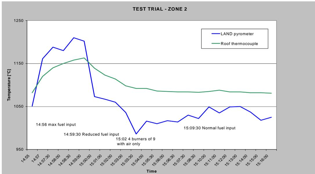
Figure 4. Test with varying burner output and furnace atmosphere at the lower measurement position in zone 2.
