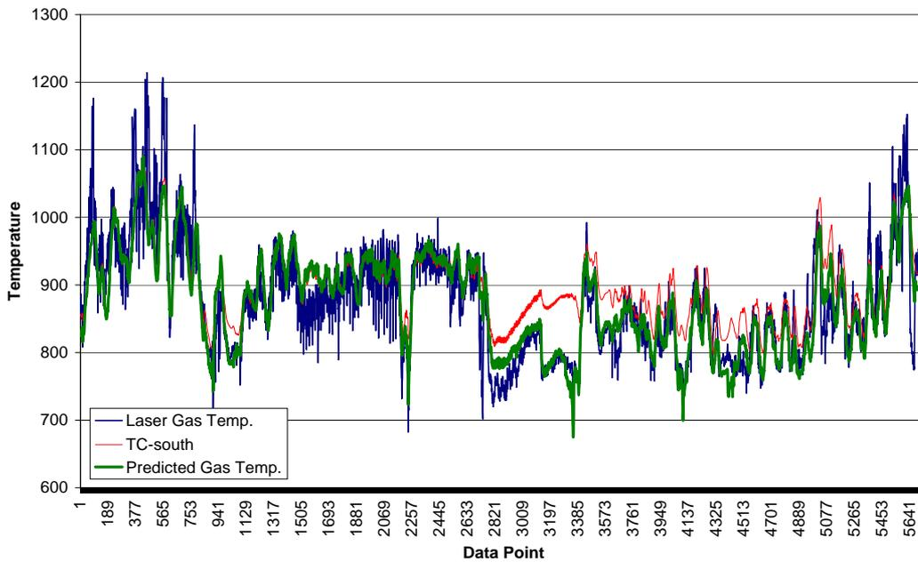
Figure 15. Predicted gas temperatures for zone 1 based on a multiple linear regression fit of the TDLAS data from December 6.
