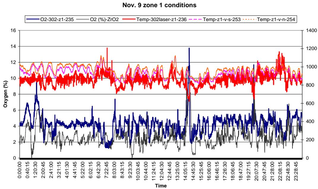
Figure 10. Good measurement stability with the TDLAS in zone 1.
