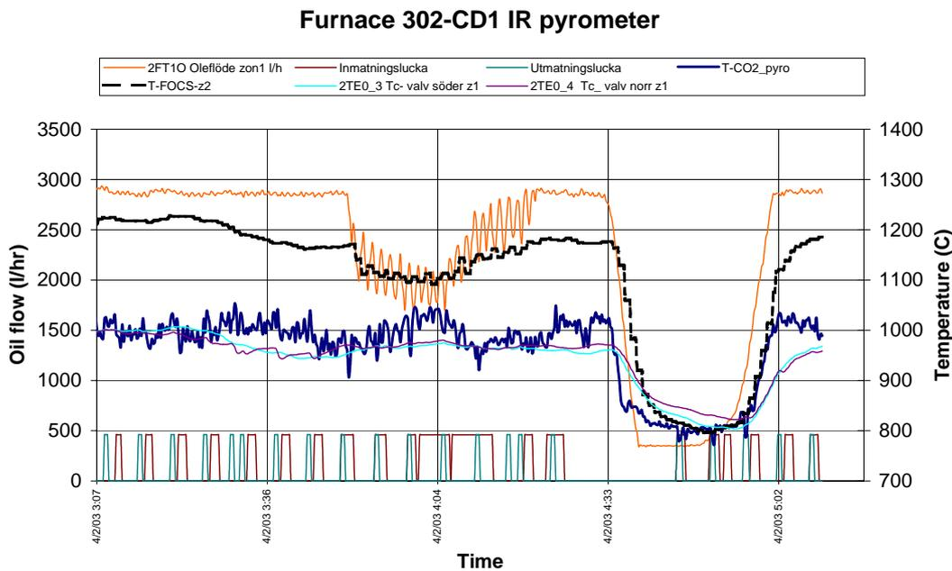
Figure 7. Deviation between FOCS and measured gas temperatures
