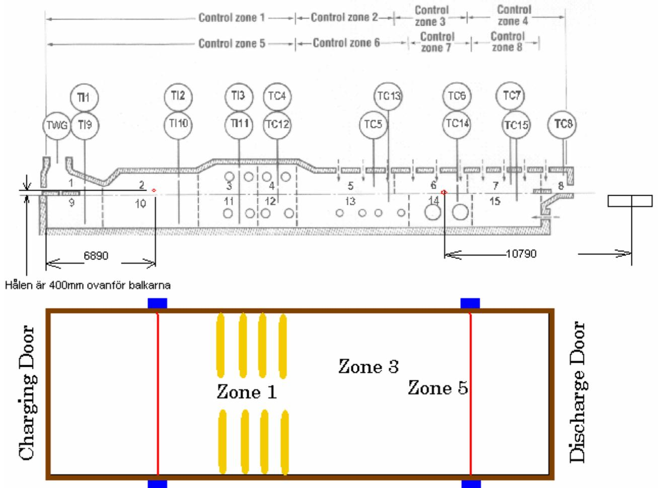
A trial to test the effect of the bowl geometry or “reflector” shape of the wall behind wall thermocouples was made at Sandvik (see the minutes of meetings 3 and 4). Various wall shapes behind the thermocouples were tested to see if there was an effect on the temperature readings. The wall shapes were not found to be important, but the penetration depth of the thermocouple was important.
