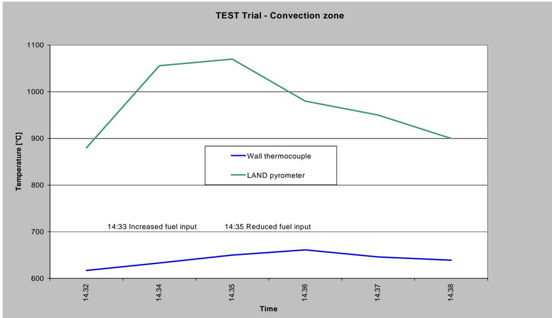
Figure 5. The effect of varying the burner outputs on the gas temperatures in the convective zone.
