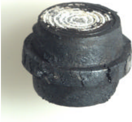
Fig.1 Hot deformed specimen of steel with 2.5%Cu after oxidation for 20s at 1100°C
