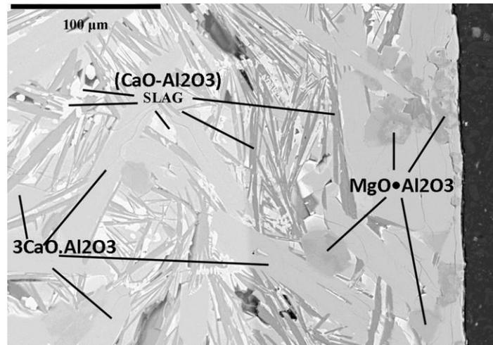
**Figure 16:** Ovako S-sample with higher magnification.
