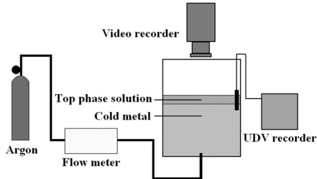
**Figure 1:** Cold model using Ga-In-Sn
