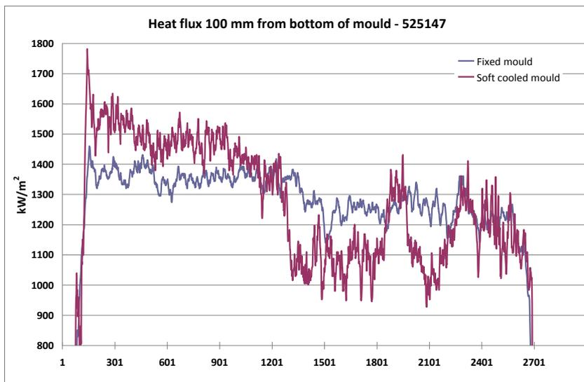
Figure 50. Heat flux at bottom of mould for carbon steel – 525147.
