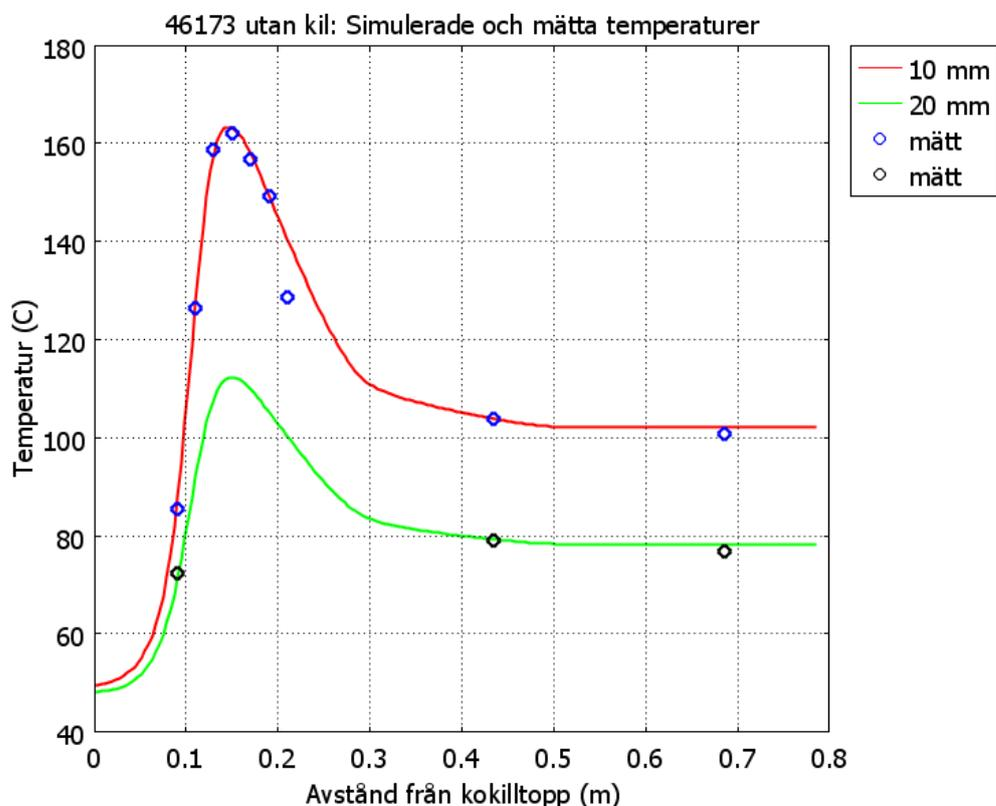
Figure 12. Measured and calculated temperatures for heat 46173.
