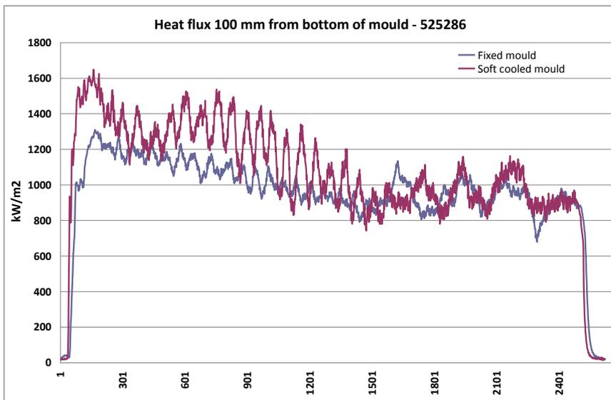
Figure 52. Heat flux at bottom of mould for stainless steel – 525286.
