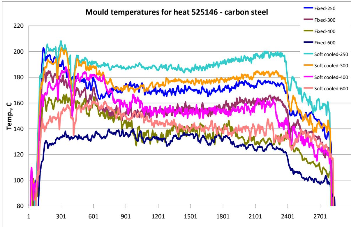
Figure 46. Mould temperatures in the middle and lower part of the mould for carbon steel 525146.
