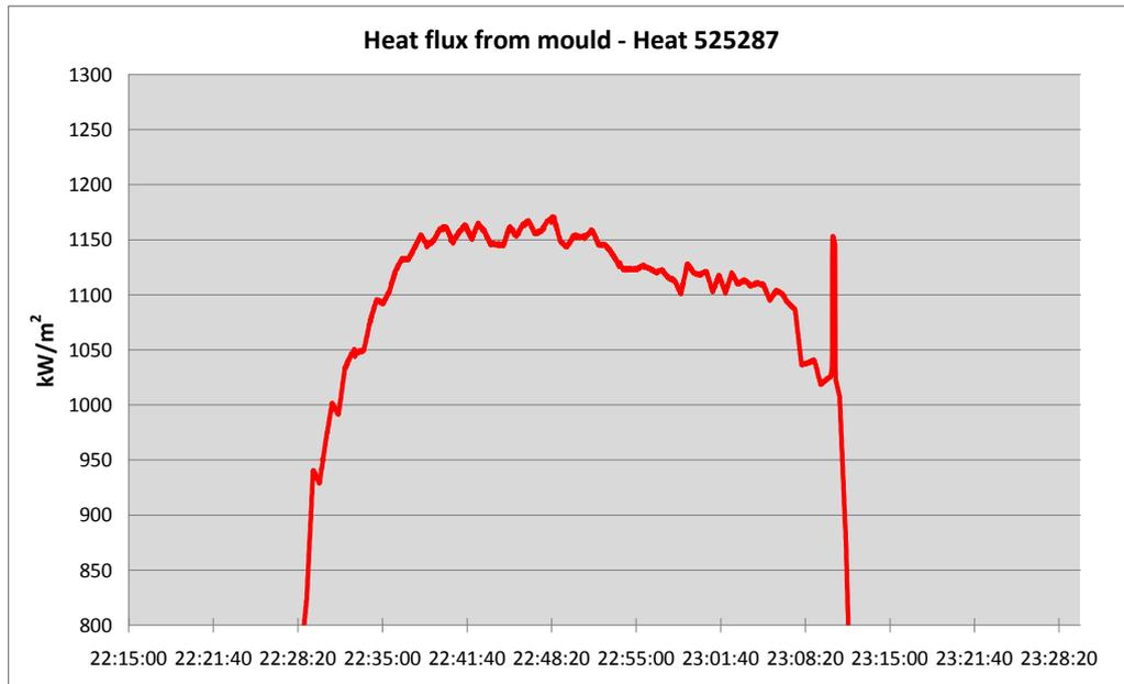
**Figure 33. Heat flux from mould in heat no. 52587.**
