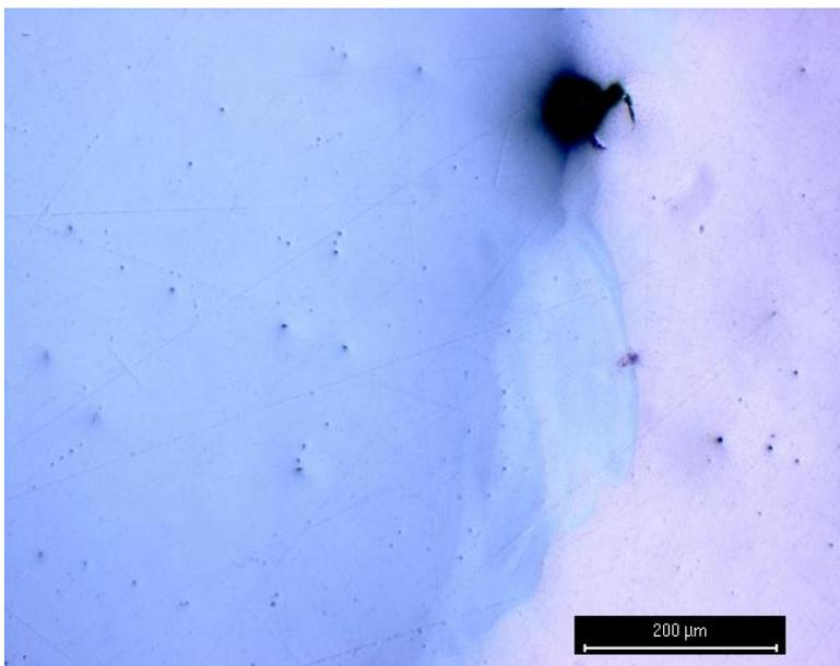
**Figure 94. LOM picture from the bonding region, 100X.**
