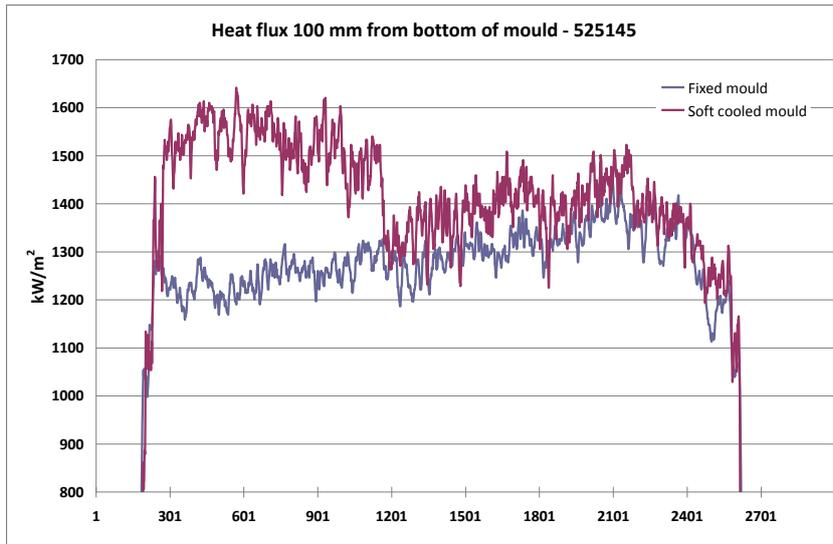
Figure 48. Heat flux at bottom of mould for carbon steel – 525145.
