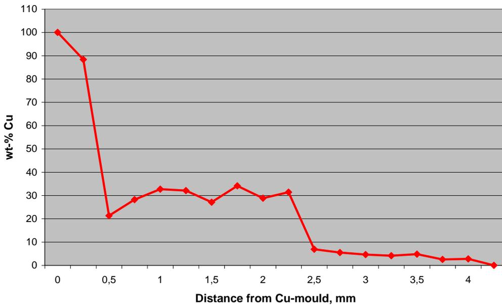
Figure 96. Cu-infiltration in Ni-weld
