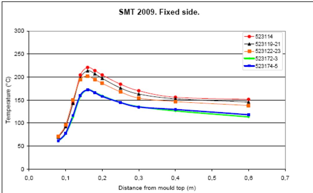
Figure 23. Mean temperatures in fixed mould for the investigated heats.
