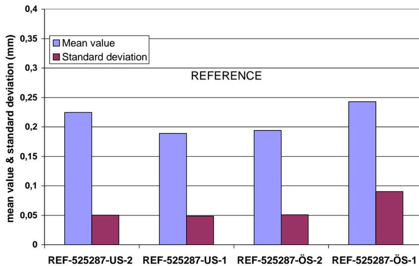
Figure 63. Relative oscillation mark depth and standard deviation for reference bloom in heat 525287.
