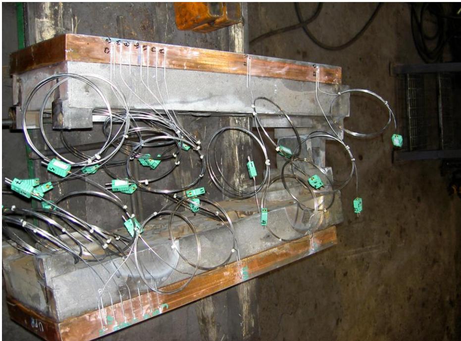
**Figure 8. Photo of mould instrumentation for the experiments at SSAB EMEA in Oxelösund.**
