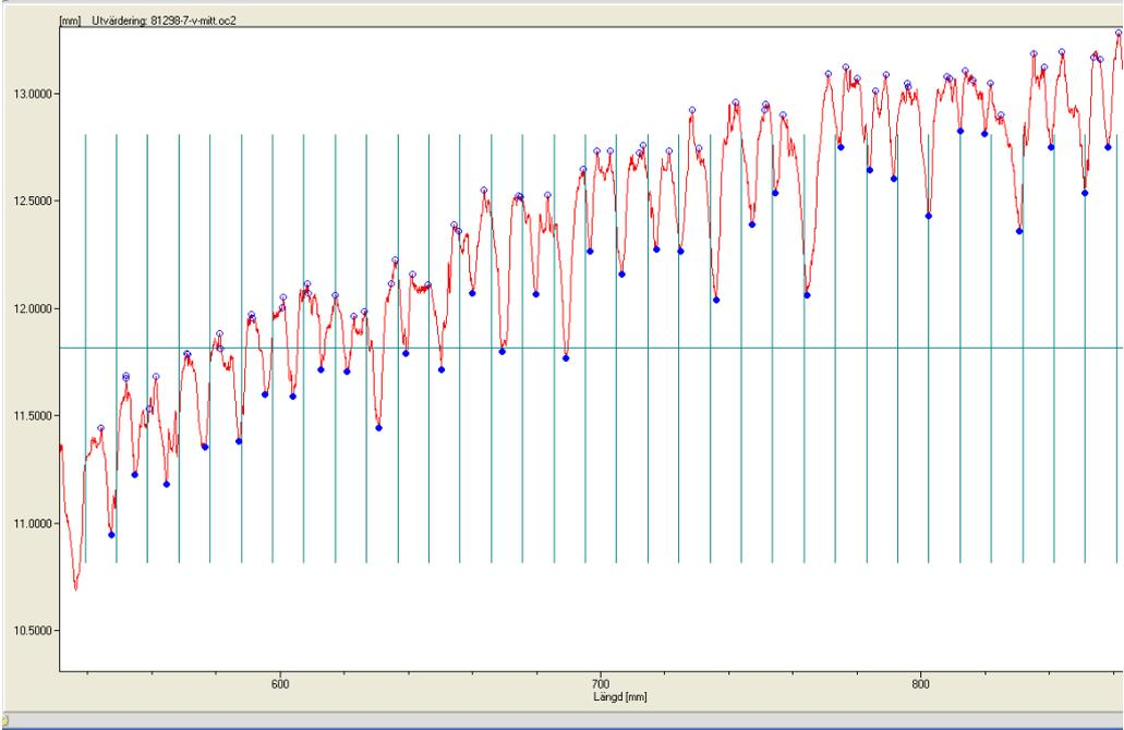
Figure 14. Surface profile with marked oscillation marks.
