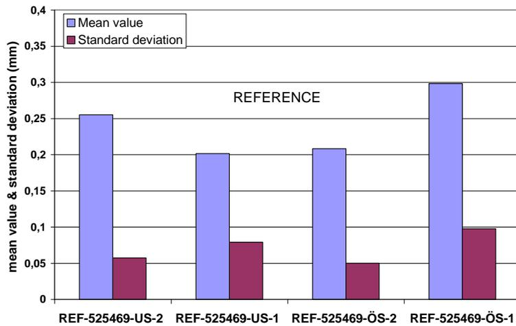
Figure 67. Relative oscillation mark depth and standard deviation for reference bloom in heat 525469.
