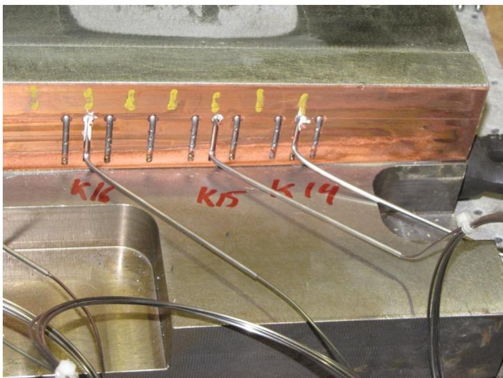
**Figure 18. Installation of mantle T.C's in the soft cooled mould.**
