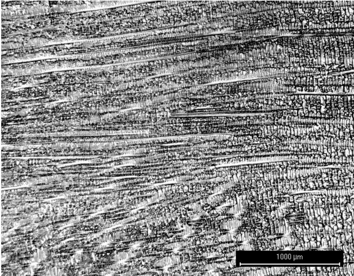
Figure 77. Structure of heat 525286 12 mm from the surface, 25X.
