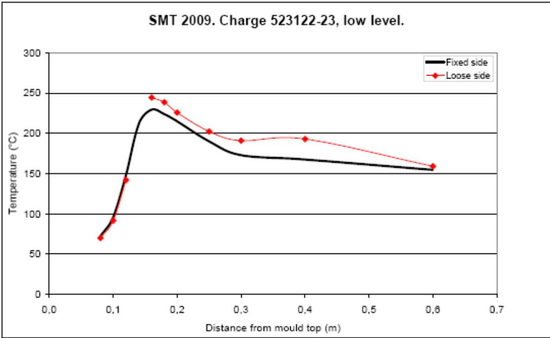
Figure 24. Mould temperatures for the carbon steel, fixed and loose side.
