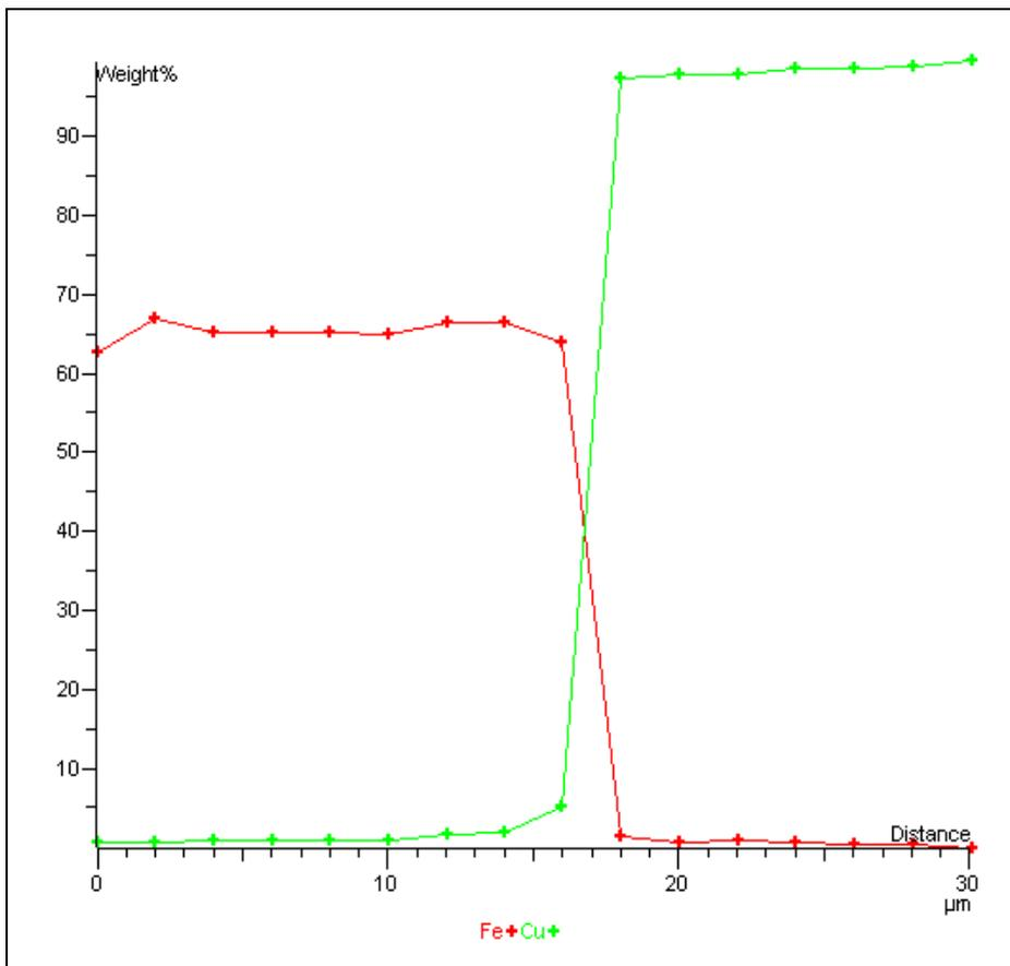
**Figure 99. Chemical composition of Fe and Cu in the bonding zone.**
