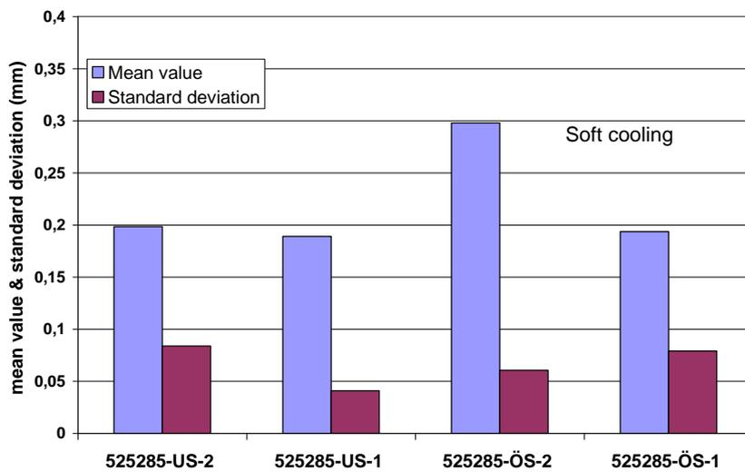
**Figure 60. Relative oscillation mark depth and standard deviation for heat 525285.**
