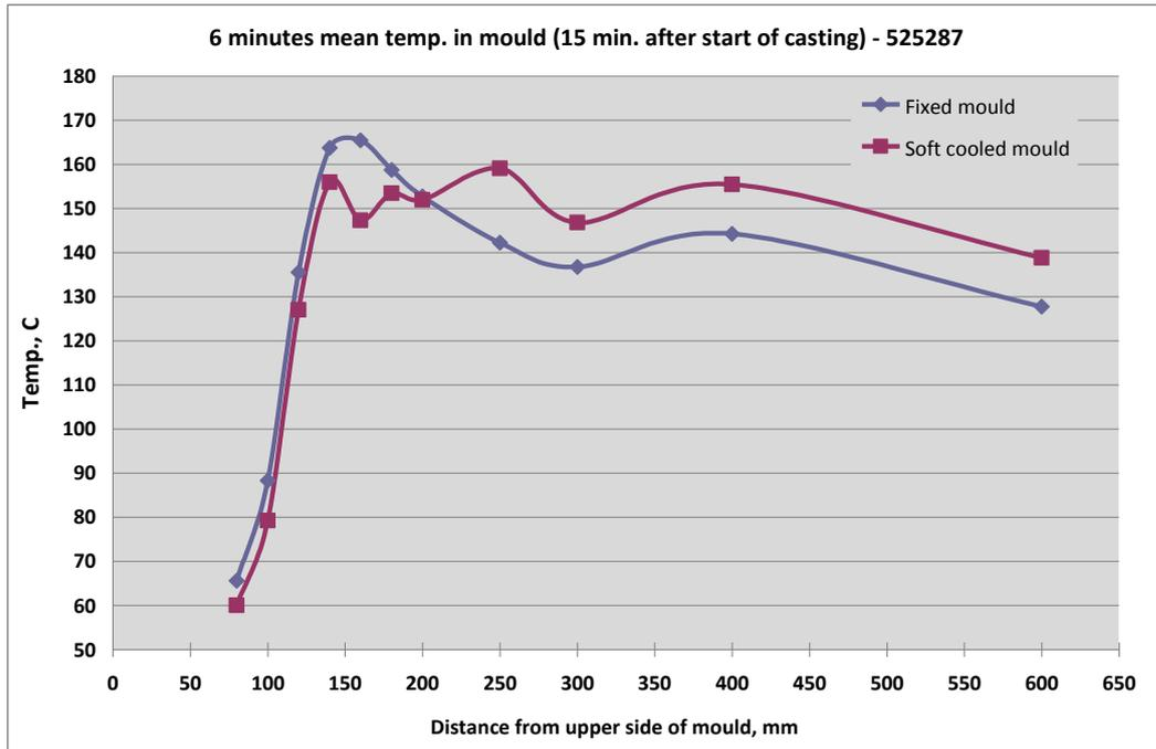
Figure 56. Mean temperatures 15 minutes from start of casting for stainless steel 525287.
