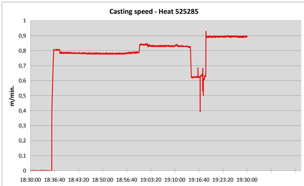
**Figure 30. Casting speed for heat no. 525285.**
