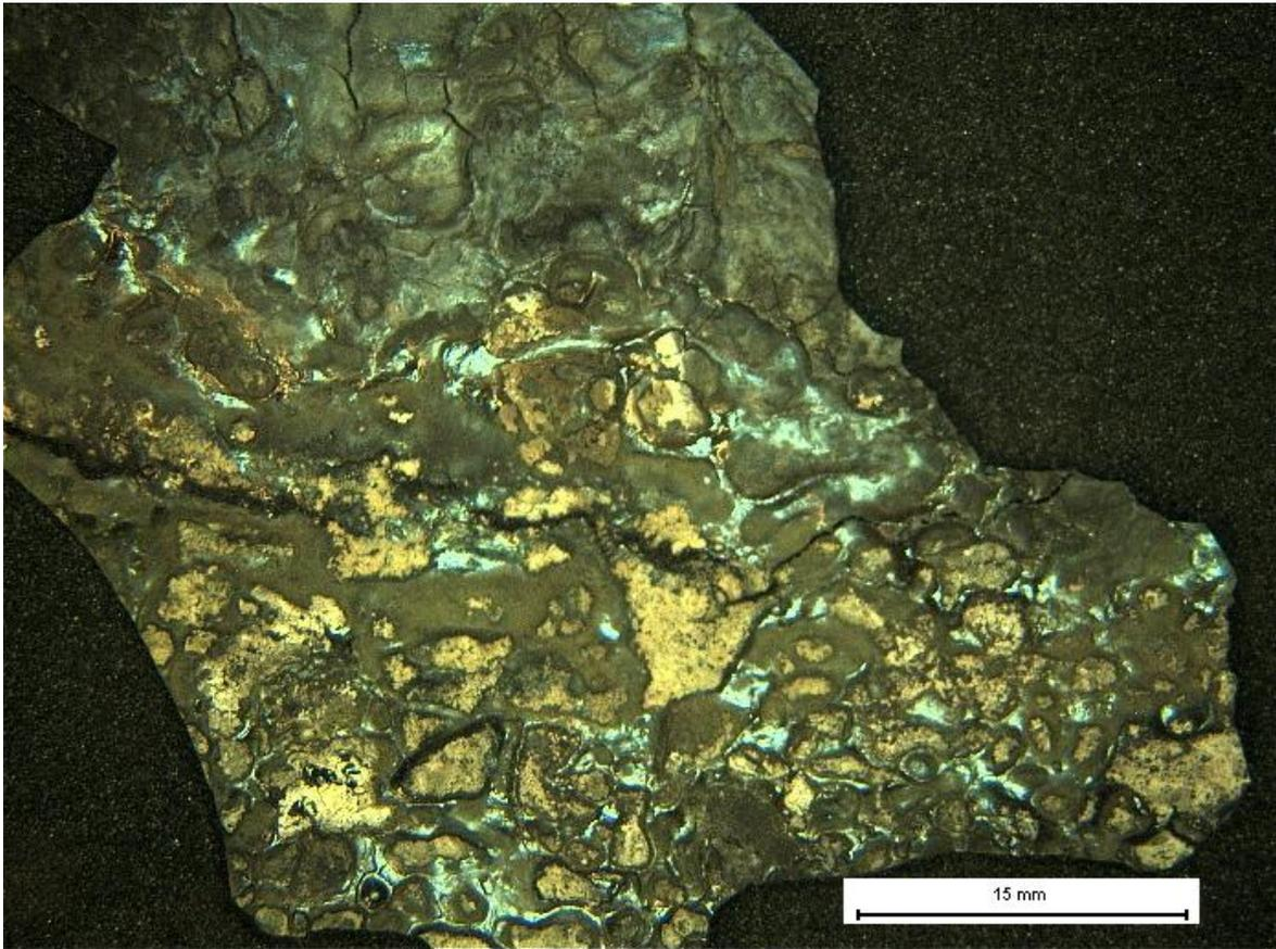
Figure 39. Surface against mould for slag film in Figure 36.
