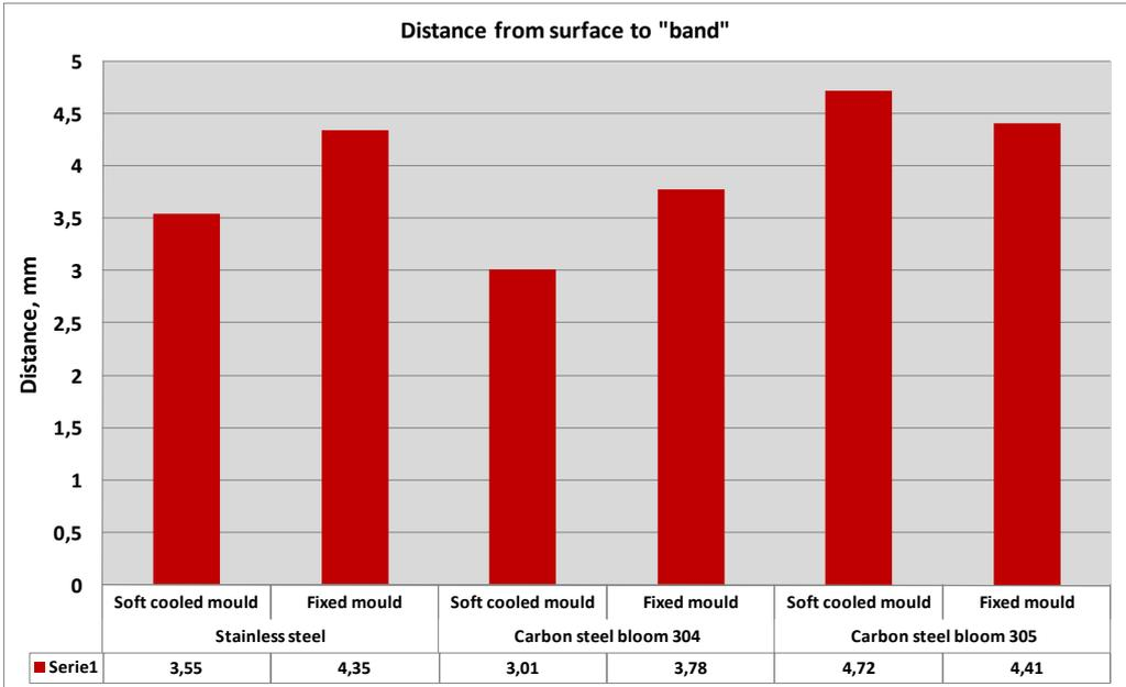
Figure 83. Distance from surface to “band” for stainless and carbon steel.
