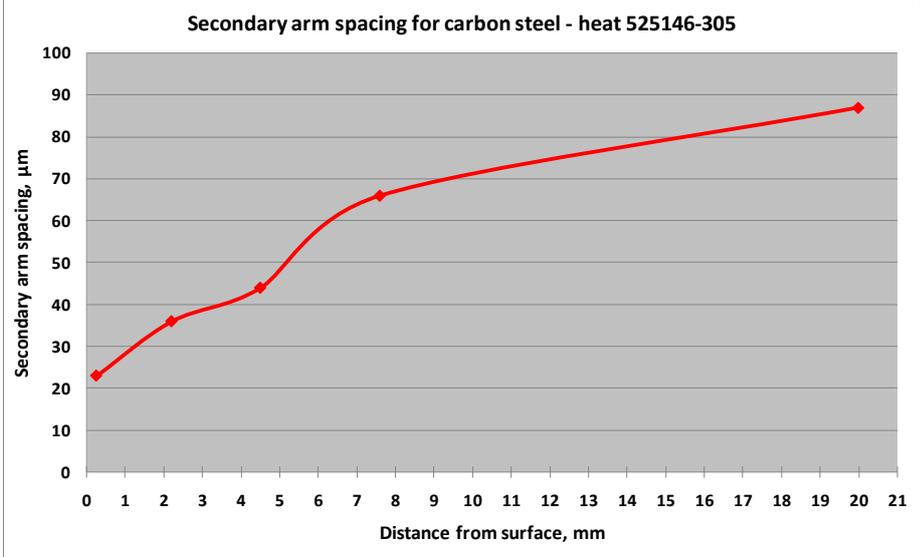
Figure 81. Secondary arm spacing for heat 525146-305 soft cooled mould.
