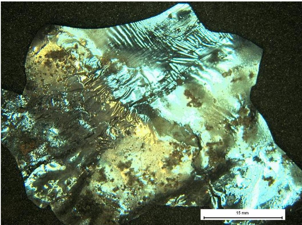
Figure 38. Surface against steel shell for slag film in Figure 36.
