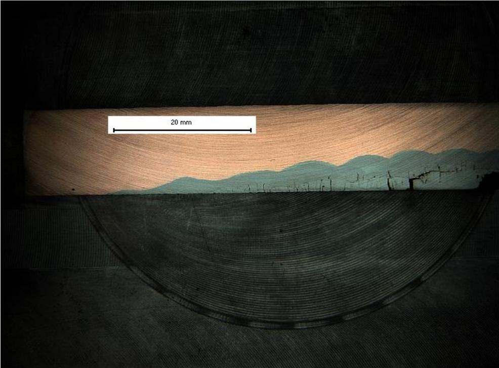
Figure 85. Photo from cross section of the weld at the lower part of the welding, 2X.
