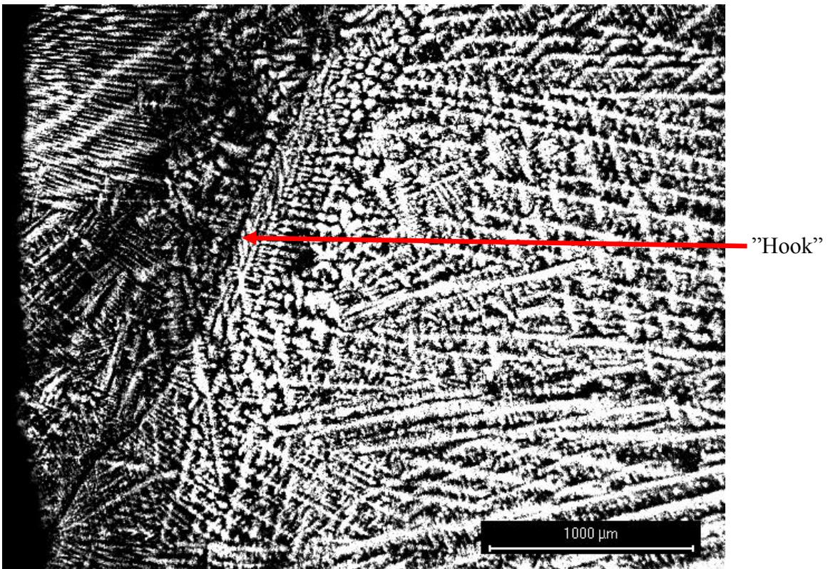
Figure 79. Example of surface area with “hook” for the fixed side of heat 525146-305.
