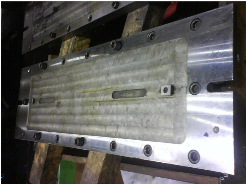
**Figure 28. Bottom steel plate needed to avoid deformation of the copper mould during welding.**
