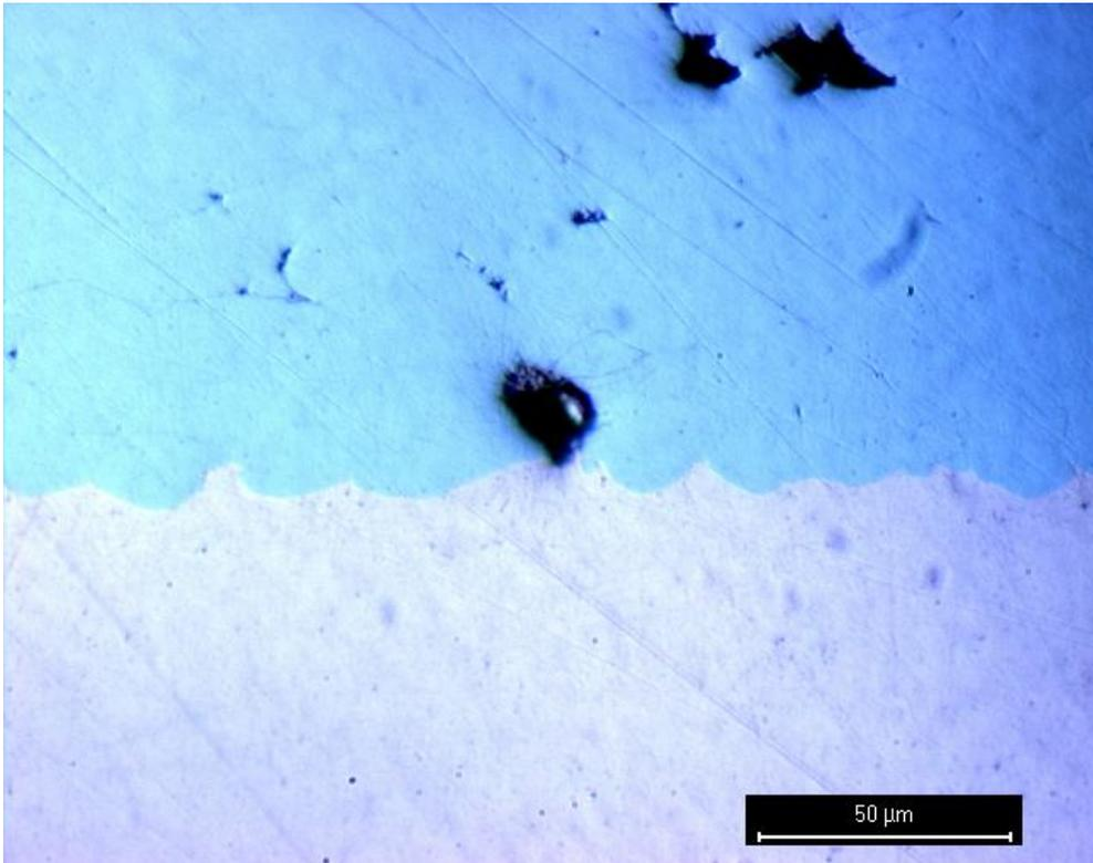
Figure 103. LOM photo from the bonding area from the cold sprayed mould, 400X.
