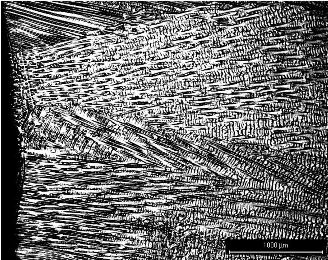
Figure 70. Surface of the stainless steel, fixed mould side, 25X.
