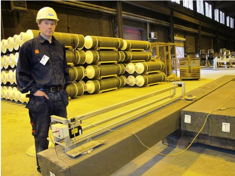
Figure 58. Johan Lönnqvist from Swerea KIMAB with the profile measurement device.
