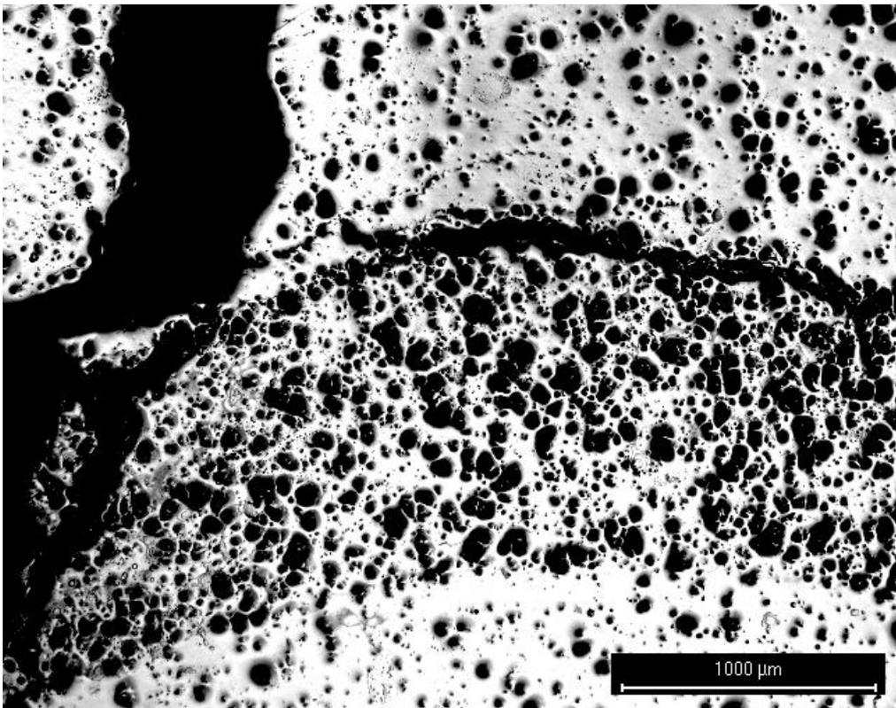
Figure 104. Photo of cracked area with stainless steel, 25X.
