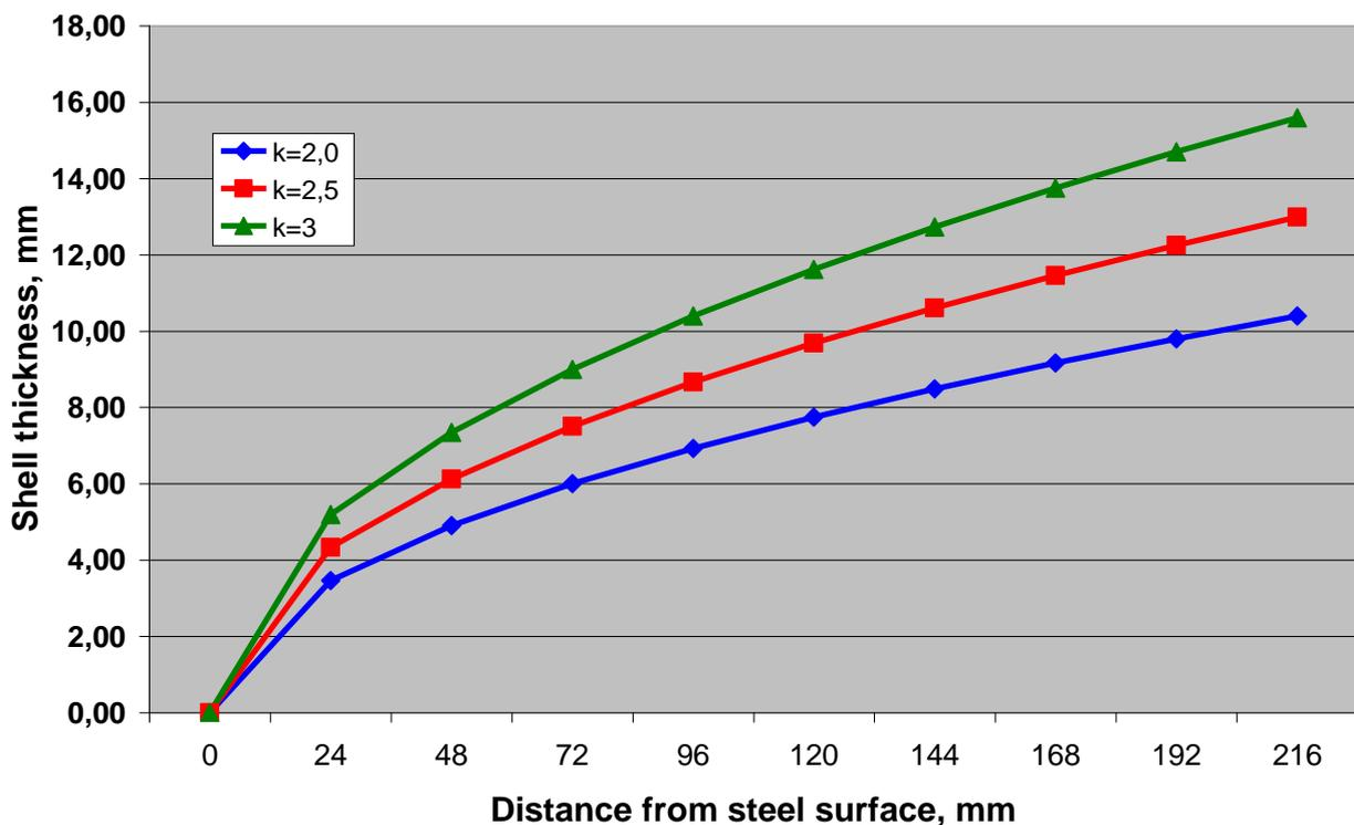
Figure 69. Calculated shell thickness according to the rule of thumb for different solidification constants.
