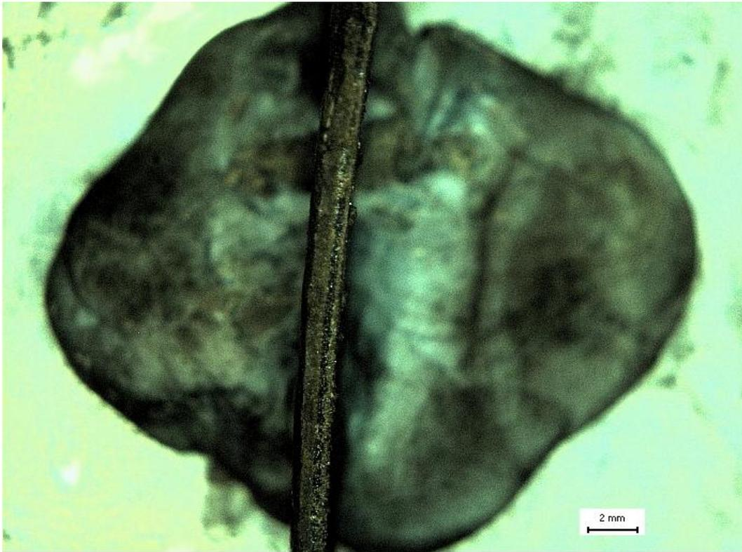
Figure 37. Cross section from slag film lower down the mould.
