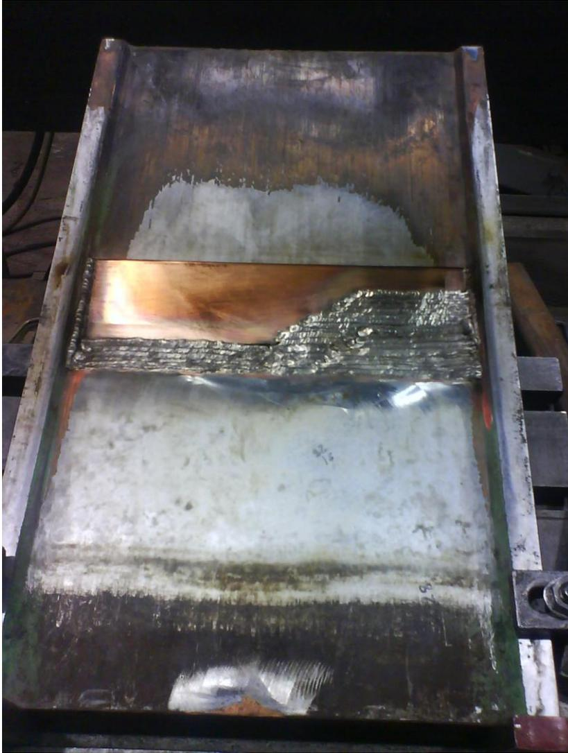
**Figure 27. Wide face mould during welding operation.**
