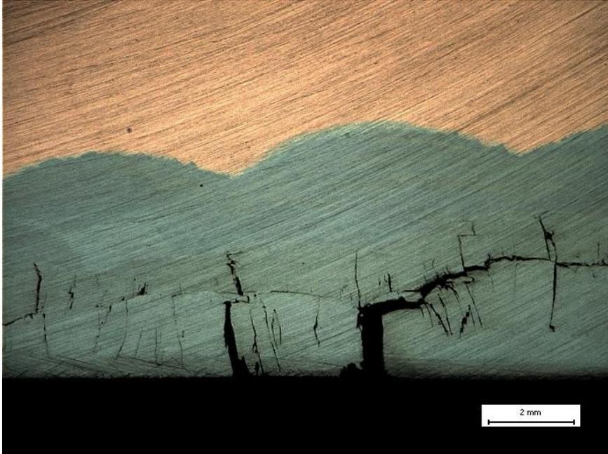
**Figure 86. Detailed photo from cross section of the weld 55 mm from steel meniscus, 10X.**
