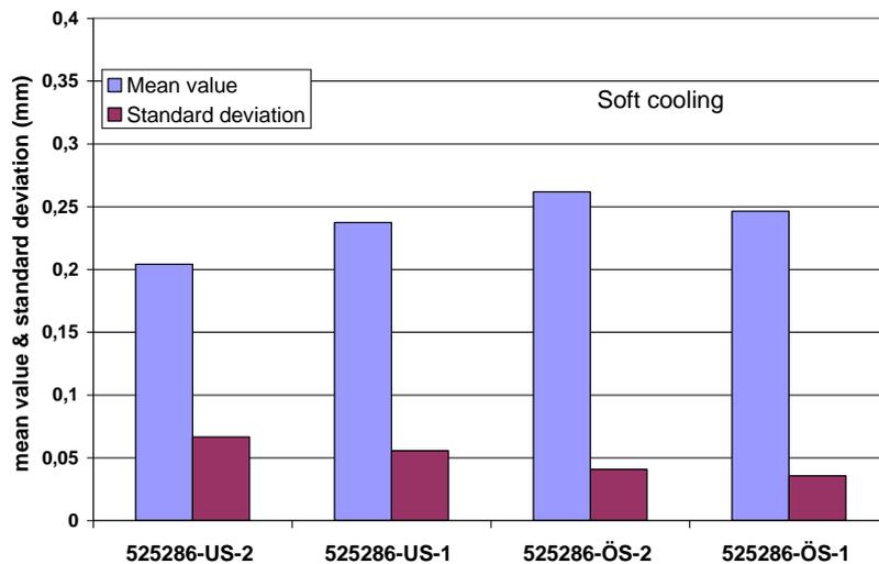
**Figure 61. Relative oscillation mark depth and standard deviation for heat 525286.**
