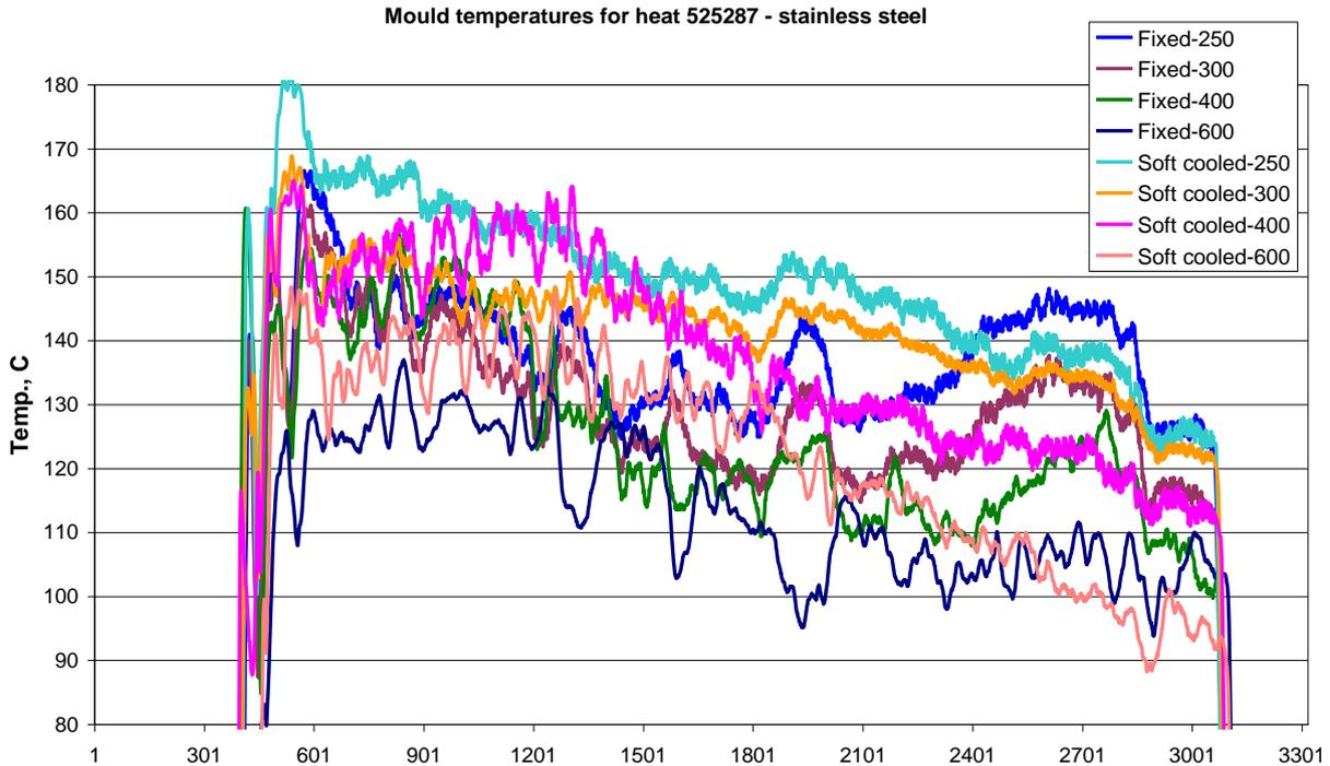
**Figure 47. Mould temperatures in middle and lower part of the mould for stainless steel 525287.**
