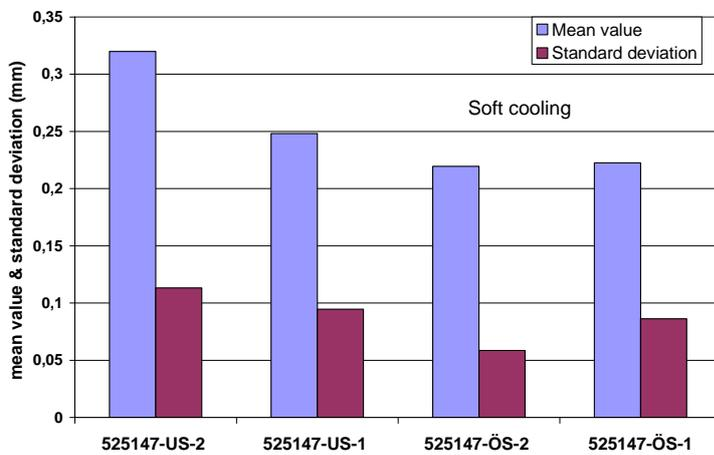
Figure 66. Relative oscillation mark depth and standard deviation for heat 525147.
