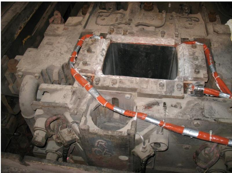
Figure 20. Instrumented mould with T.C. cables.
