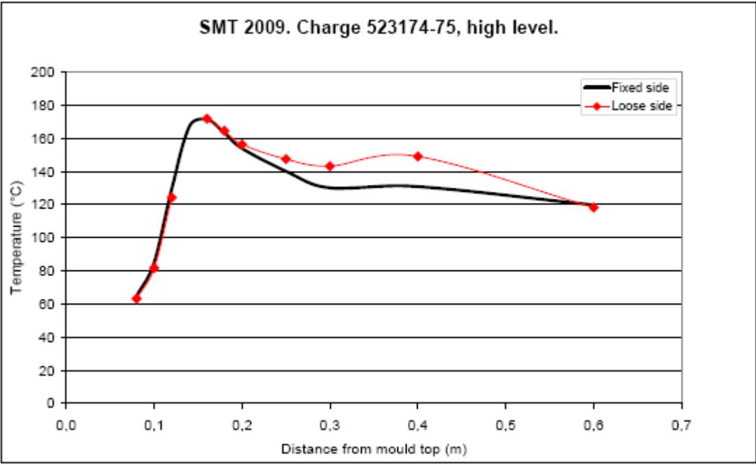
Figure 25. Mould temperatures for the stainless steel, fixed and loose side.
