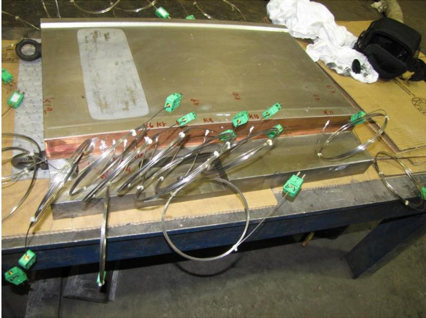
Figure 19. Soft cooled mould mantled with 18 T.C's.
