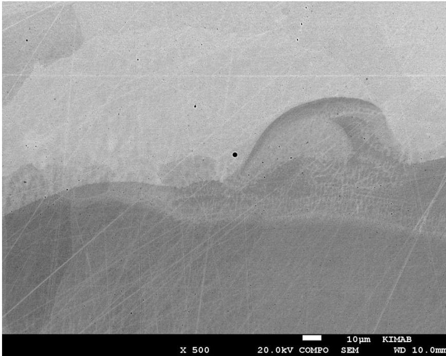
Figure 95. SEM picture of the bonding, 500X.
