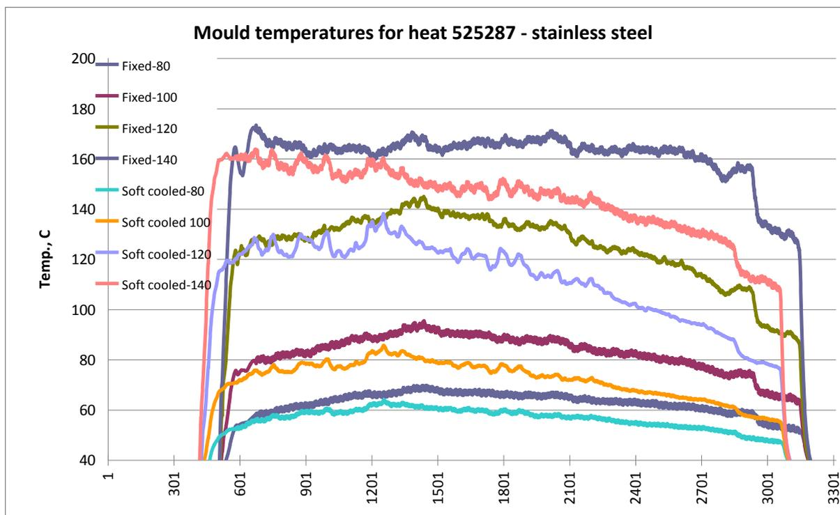
Figure 45. Mould temperatures in the upper part for stainless steel heat 525287.
