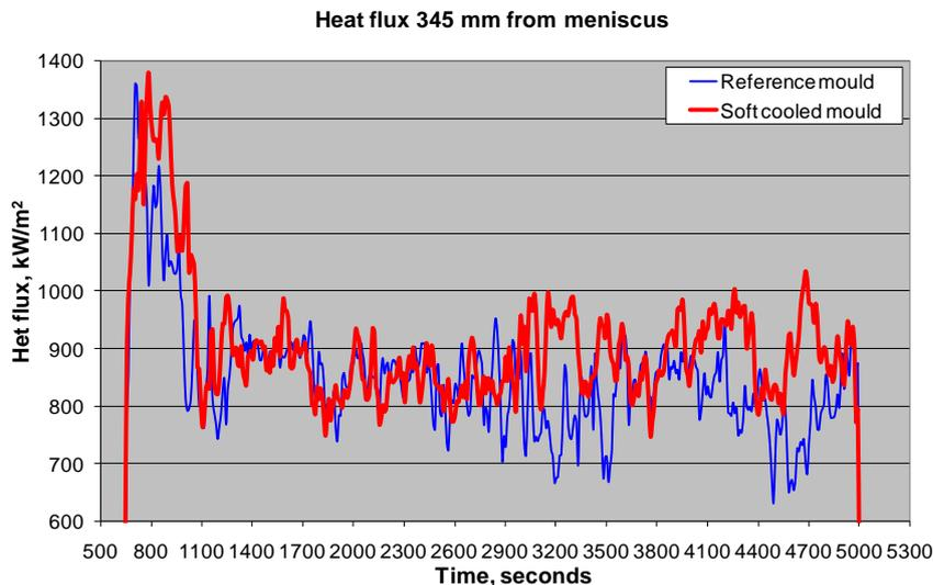
Figure 11. Heat flux 345 mm from meniscus for heat 46173.
