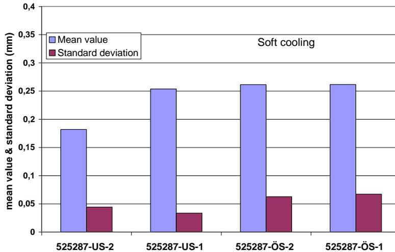
Figure 62. Relative oscillation mark depth and standard deviation for heat 525287.
