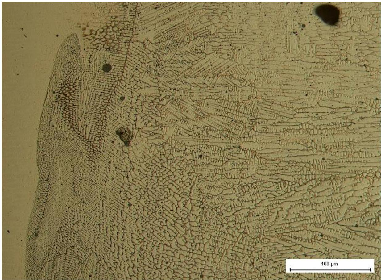
**Figure 87. Contact area between Ni-layer and 253 MA, 200X.**
