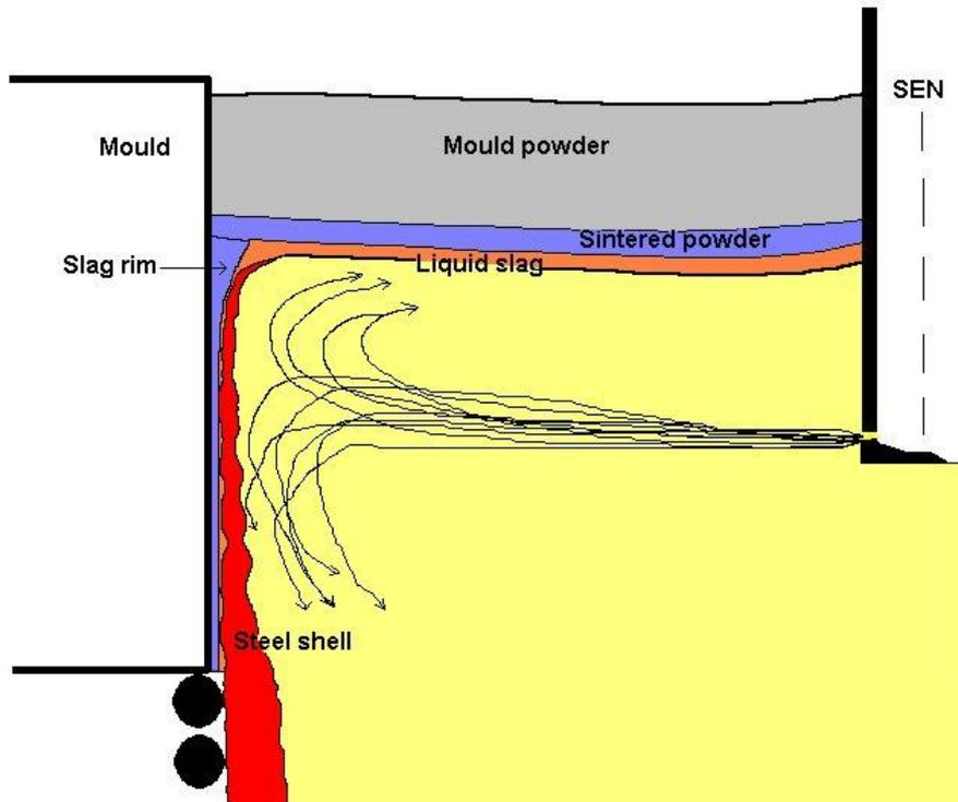
Figure 2. Schematic picture of CC mould for a slabs machine (half width).
