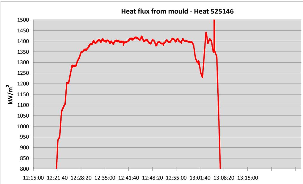
**Figure 32. Heat flux from mould in heat no. 525146.**
