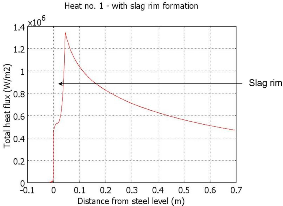
**Figure 73. Calculation of heat flux exemplifying the strong influence of the slag rim [ref. 16].**
