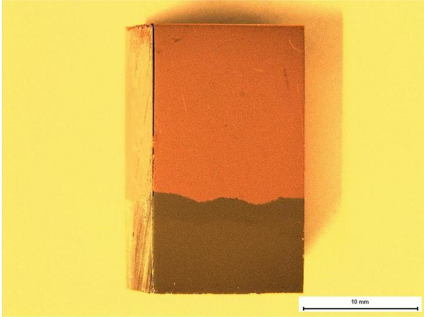
**Figure 93. Macro photo of cross section with Ni weld.**
