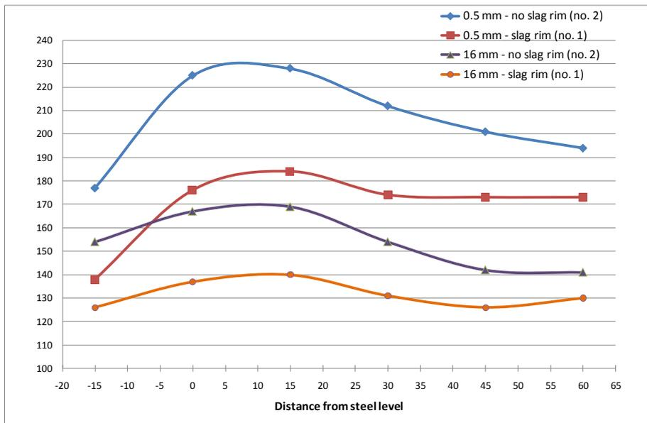
**Figure 74. Temperature measurements in the meniscus area, with and without slag rim [ref. 16].**
