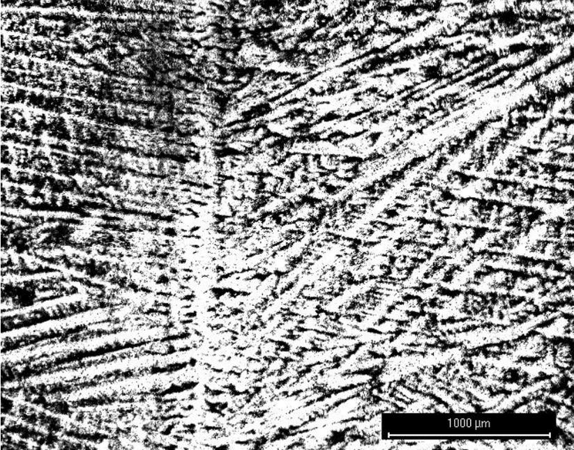
Figure 80. Photograph 4 mm from the surface of the fixed mould for heat 525146-305, 25X.
