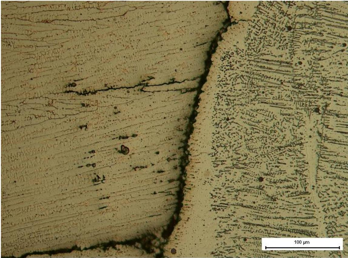
Figure 88. Bonding zone between two welding layers with cracking, 200X.
