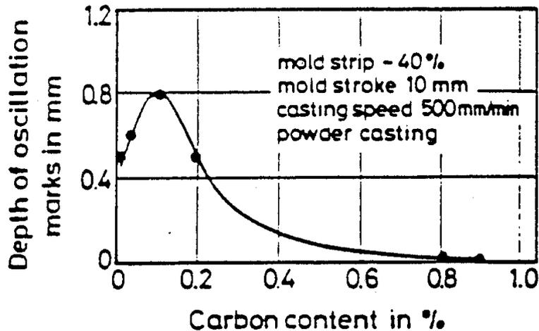
Figure 17. Oscillation mark depth as a function of carbon content [ref. 10]
