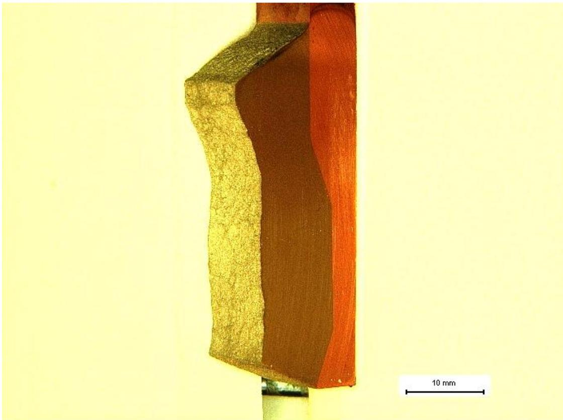
Figure 97. Cross section of a “cold sprayed” layer of stainless steel on copper.
