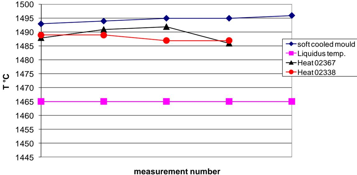
Figure 106. Tundish temperature for test- and reference heats.
