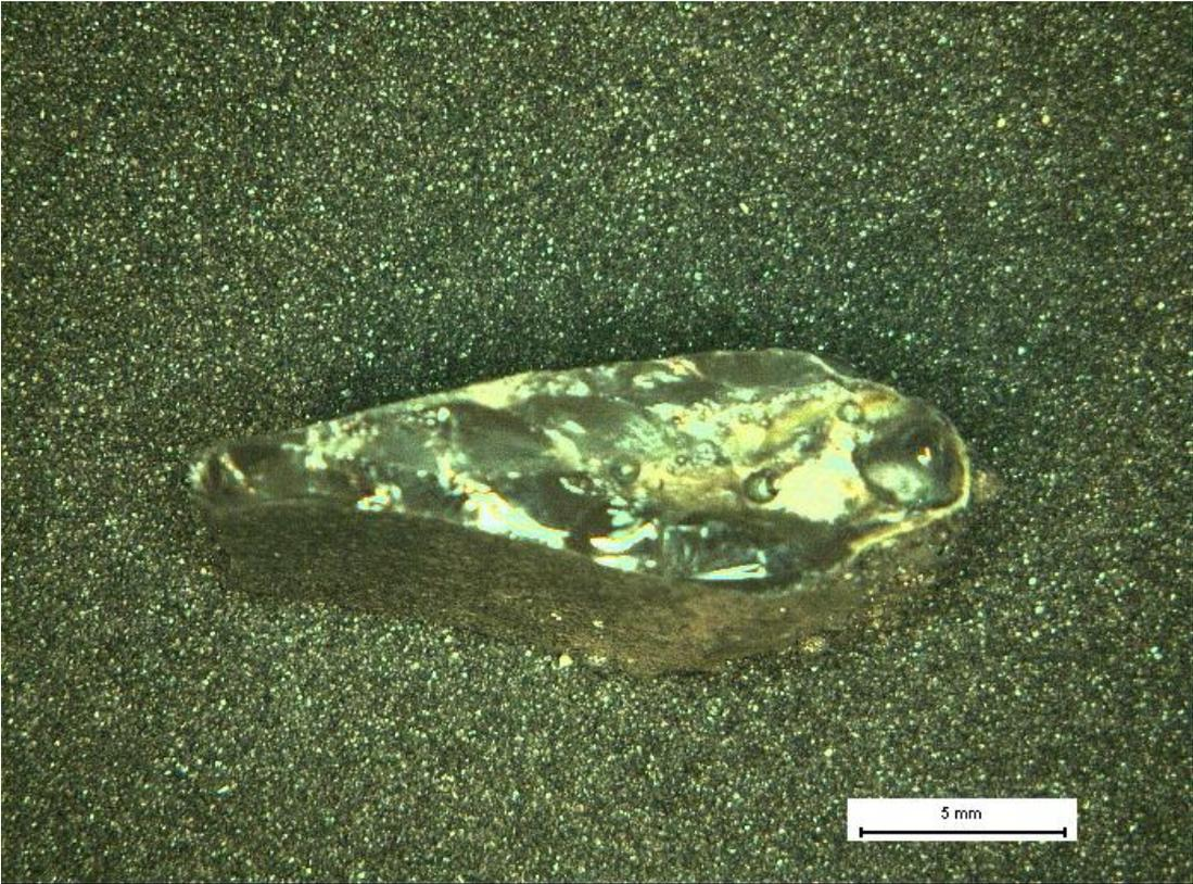
Figure 40. Slag rim partly crystallised in the upper part.
