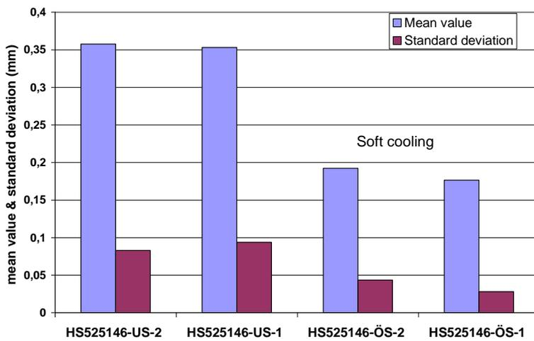
Figure 65. Relative oscillation mark depth and standard deviation for heat 525146.
