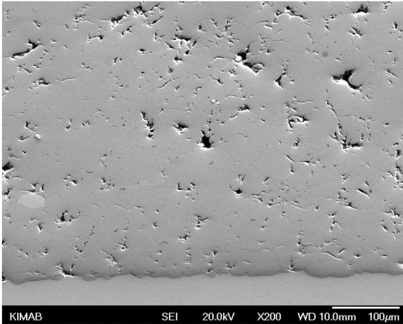
**Figure 98. Bonding area with cold sprayed stainless steel against copper, 200X.**
