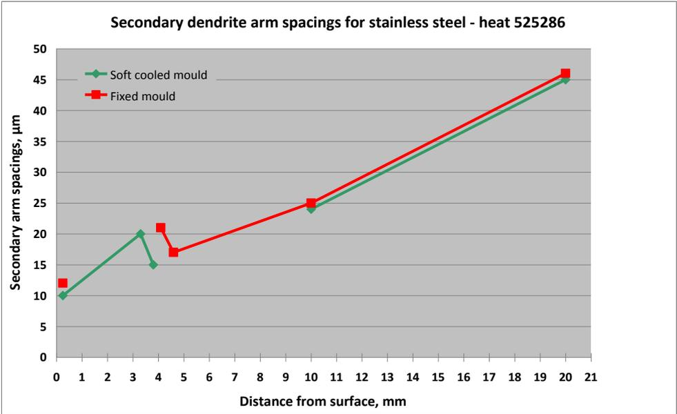
Figure 76. Secondary arm spacing for stainless steel heat 525286.
