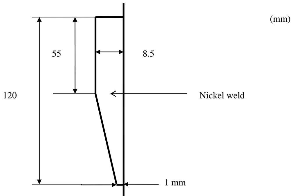
Figure 26. Dimensions of the nickel wedge for soft cooling.
