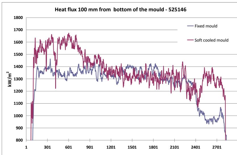
Figure 49. Heat flux at bottom of mould for carbon steel – 525146.
