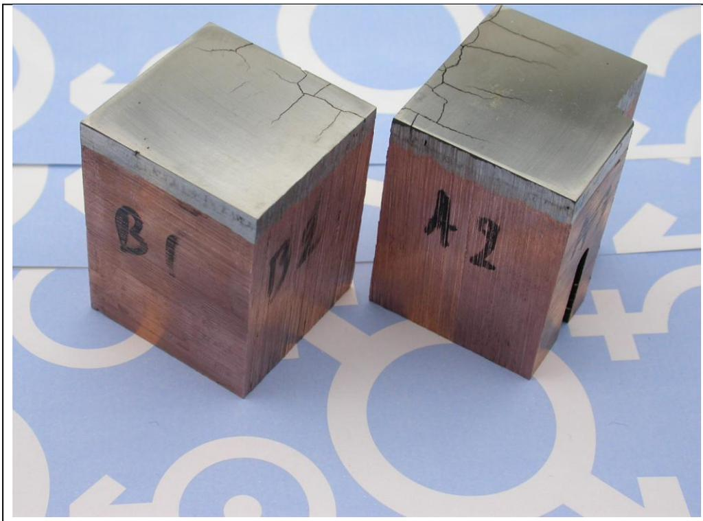
Figure 90. Samples for investigation of thermal conductivity with hot disk.
