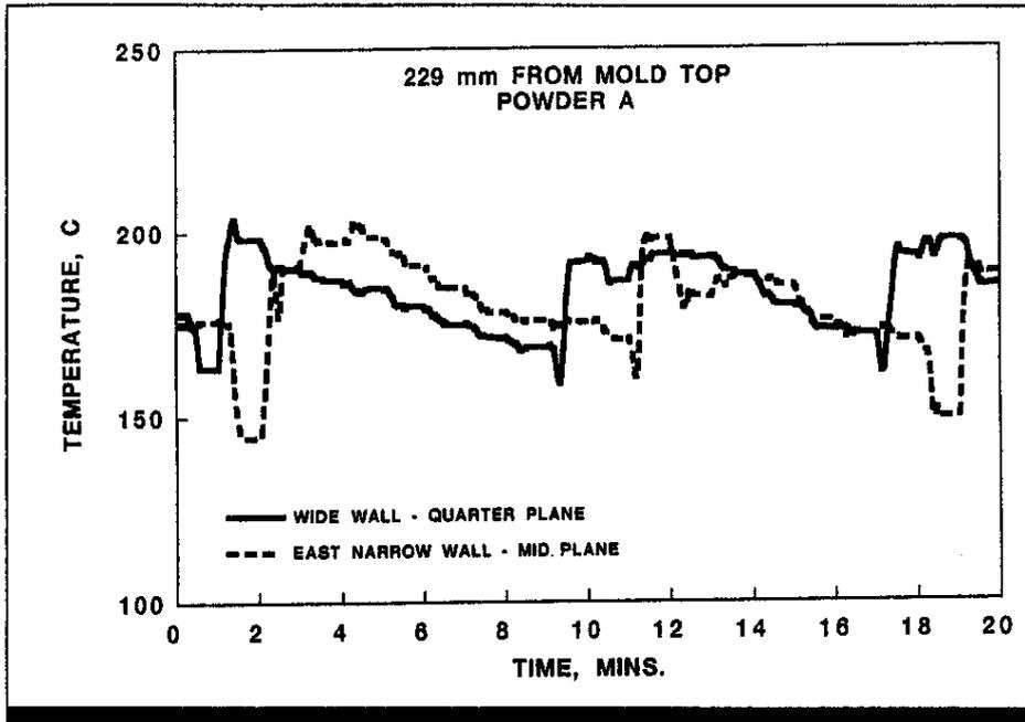
Figure 4. Temperature measurements in mould for a casting with a 1.62 basicity mould powder.
