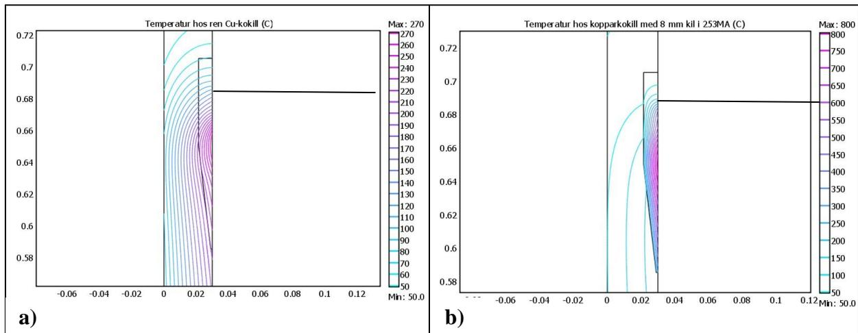
**Figure 7. Temperature distribution in a mould without (a) and with (b) a 8 mm wedge of 253 MA.**
