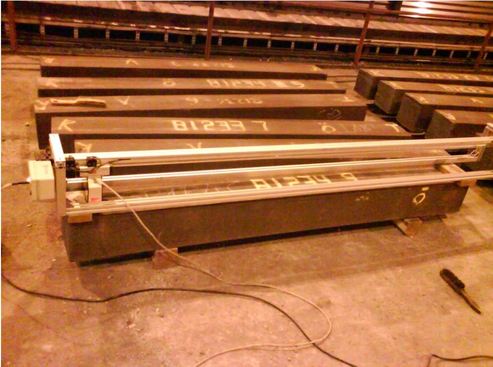
Figure 13. Swerea KIMAB's equipment for measurement of oscillation mark depth.
