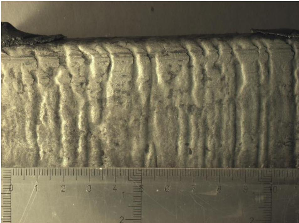
**Figure 1. Example of uneven shell formation for a peritectic stainless steel grade**
