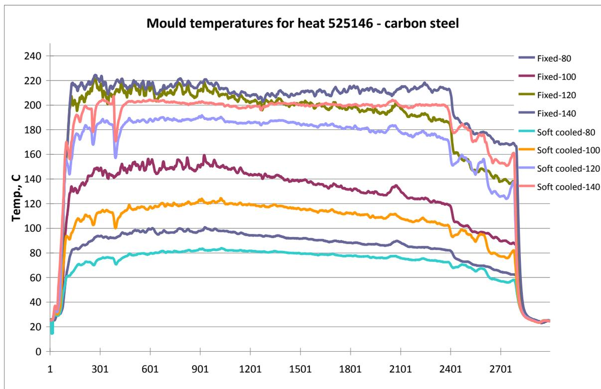
Figure 44. Mould temperatures in the upper part of the mould for carbon steel heat 525146.
