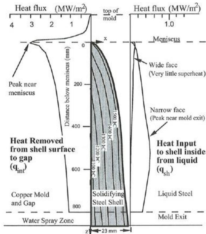
Figure 6. Heat removal from shell surface to mould [ref. 5].
