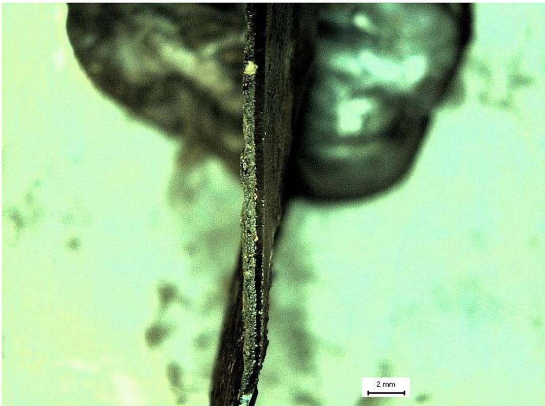
**Figure 36.** Cross section from a slag film just below the slag rim.
