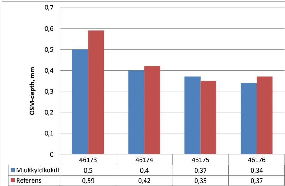
Figure 15. Results from measurements of oscillation mark depth.
