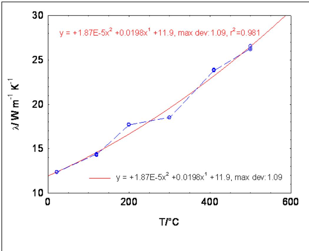
Figure 91. Results from hot disk evaluation of welded Ni-layer.
