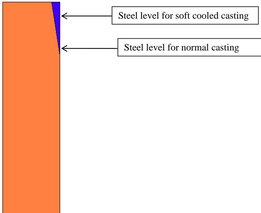
**Figure 5. Schematic drawing of the soft cooled mould concept.**
