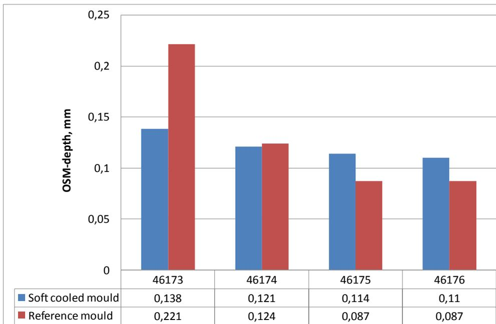
Figure 16. Standard deviation from measurements of oscillation mark depth.
