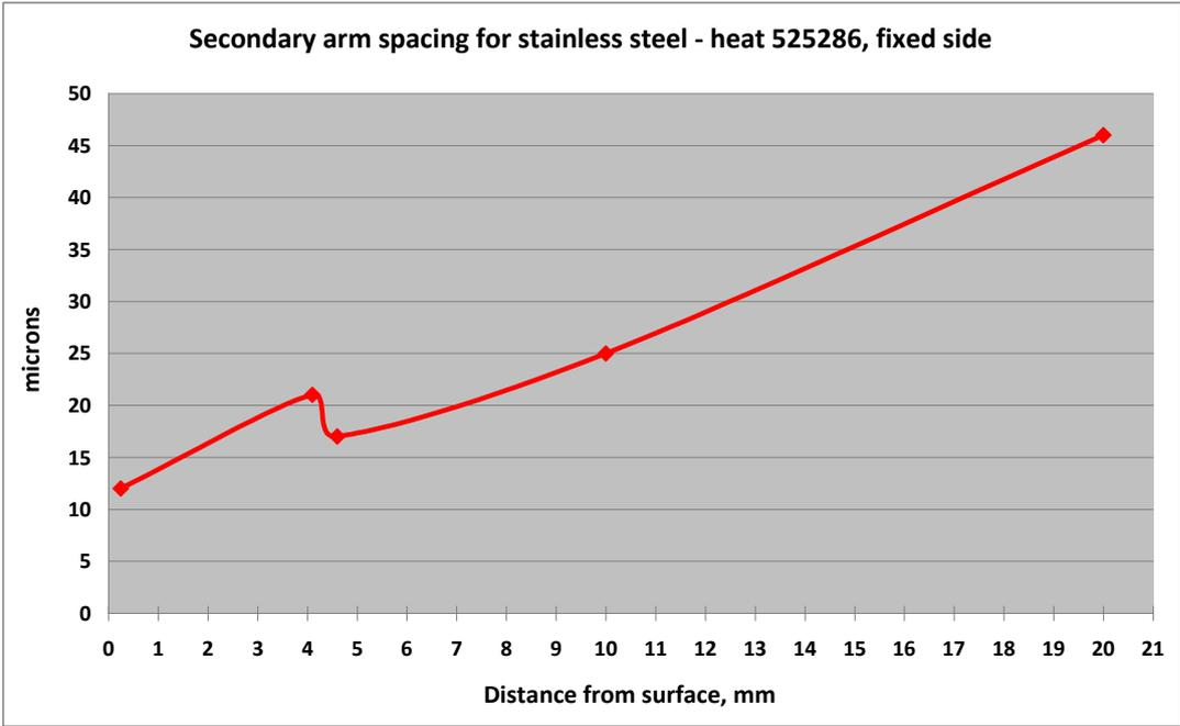
Figure 75. Secondary arm spacing for heat 525286, fixed side.
