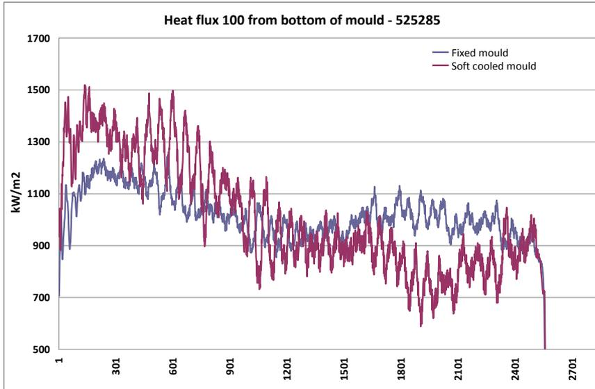
Figure 51. Heat flux at bottom of mould for stainless steel – 525285.
