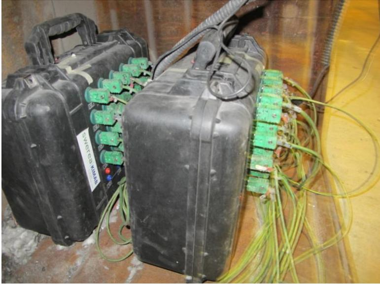
**Figure 21. Swerea KIMAB:s new equipment for data logging.**
