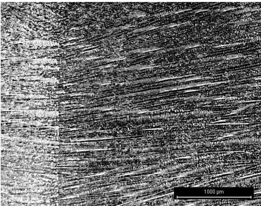
Figure 71. Photograph of “band” 4 mm from the surface of the soft cooled mould, 25X.
