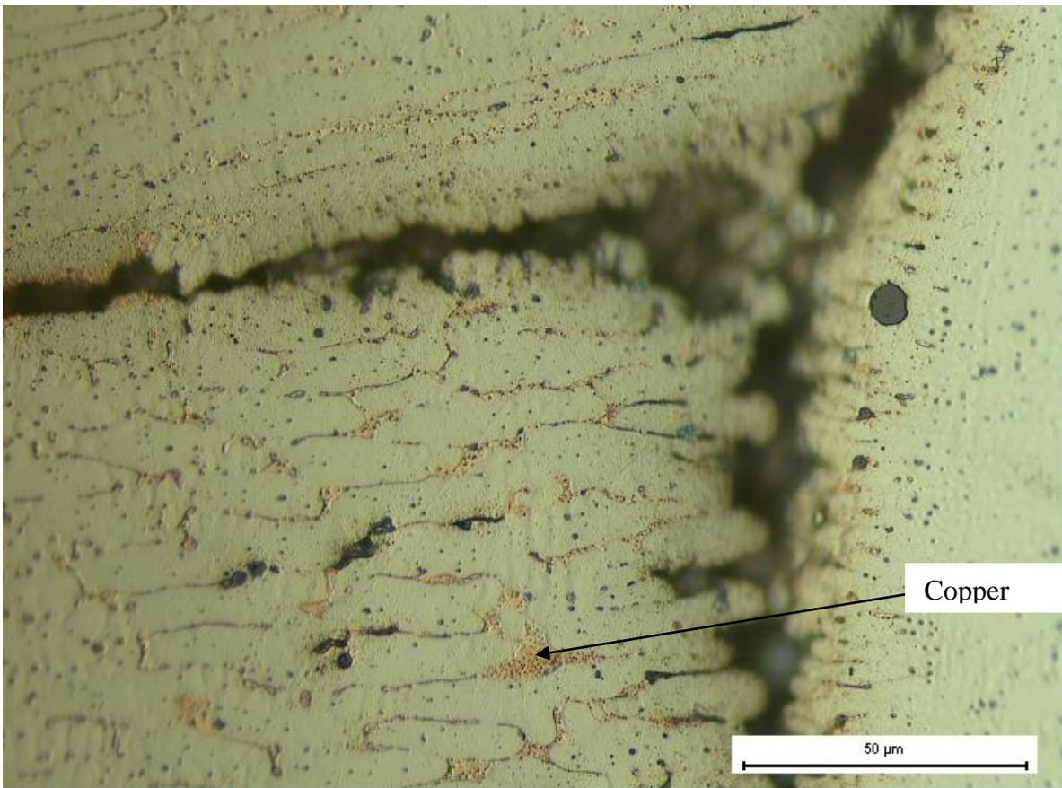
Figure 89. Bonding zone between two welding layers with cracking, 500X.
