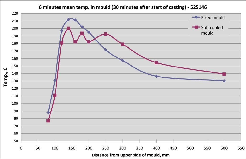
Figure 55. Mean temperatures 30 minutes from start of casting for carbon steel – 525146.
