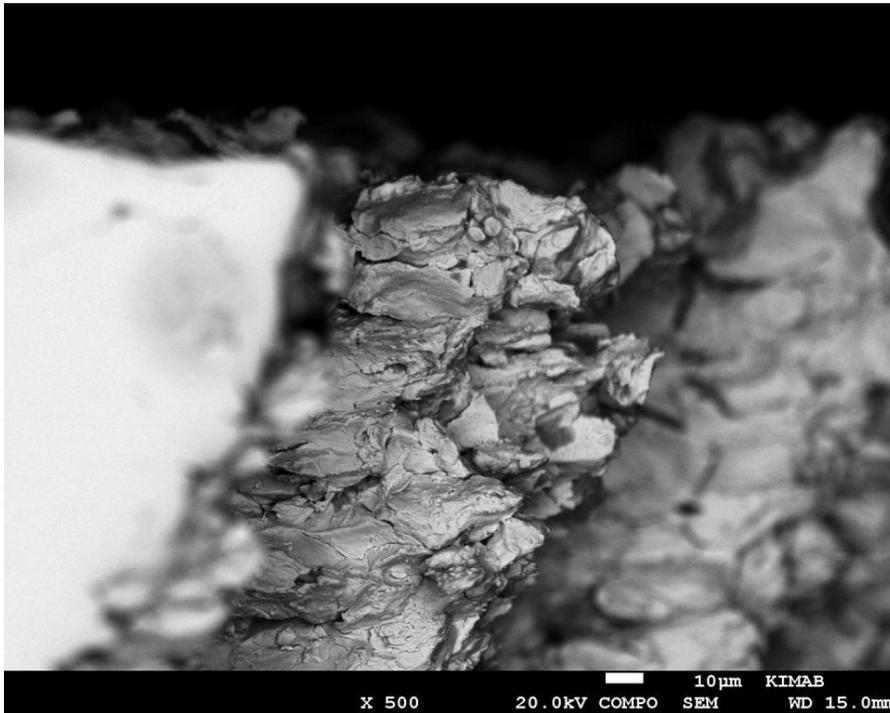
**Figure 105. SEM-picture from the crack in the stainless steel, 500X.**
