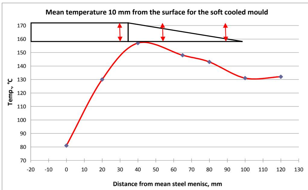
**Figure 87. Mean temperature for soft cooled mould for heat 46176.**
