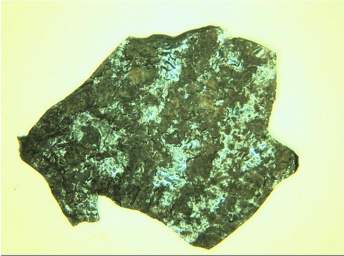
**Figure 42. Surface against mould for slag film in Figure 41.**
