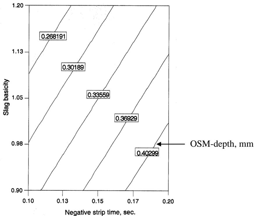
Figure 68. Oscillation mark depth as a function of slag basicity and negative strip time [reg. 15].
