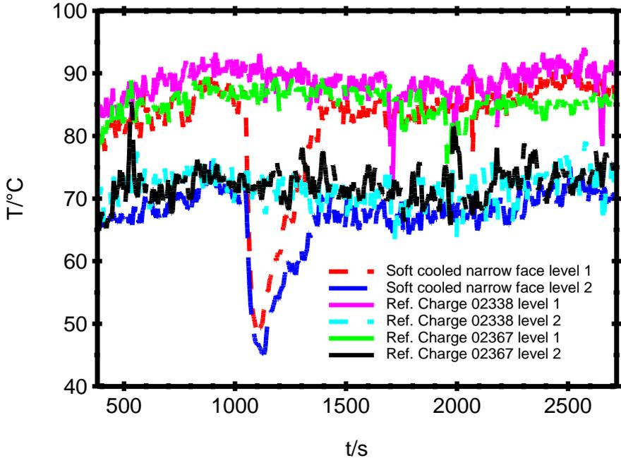
Figure 107. Temperatures from thermocouples in soft cooled mould and in a reference heat.
