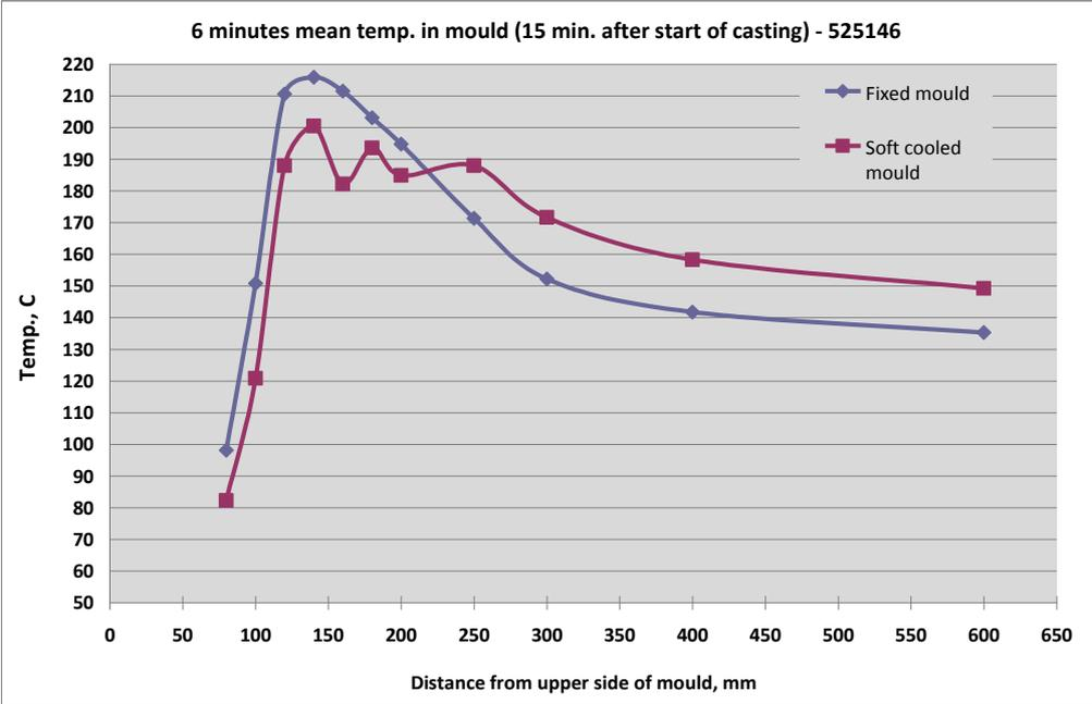
Figure 54. Mean temperatures 15 minutes from start of casting for carbon steel – 525146.
