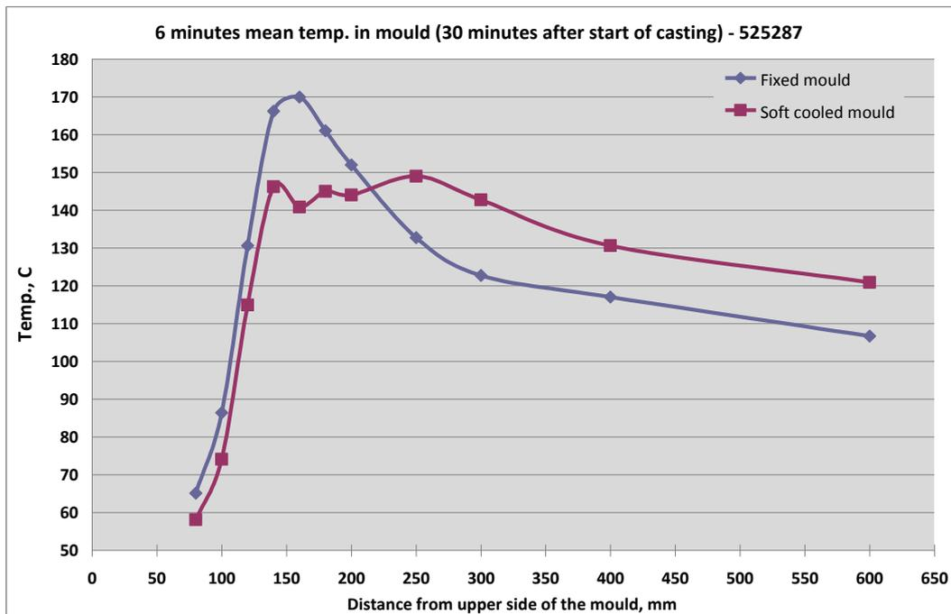
Figure 57. Mean temperatures 30 minutes from start of casting for stainless steel 525287.
