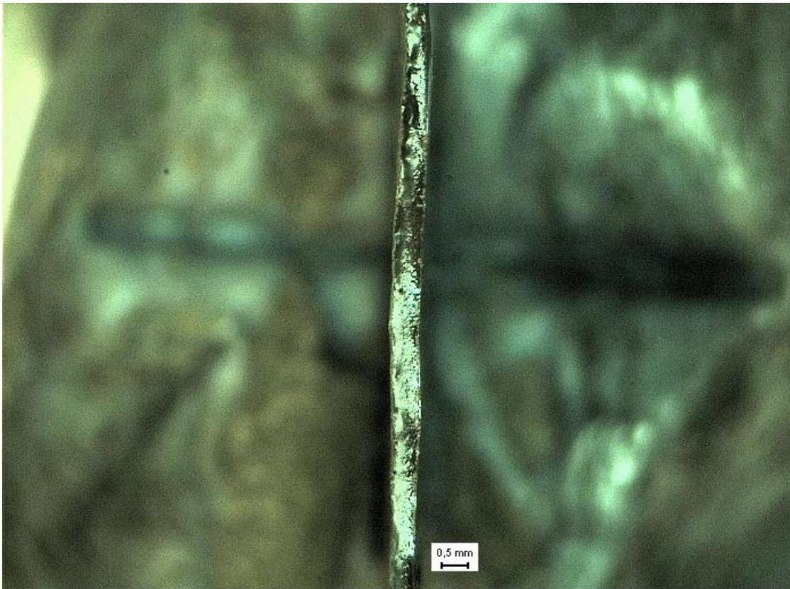
**Figure 43. Cross section of slag film further down the mould.**
