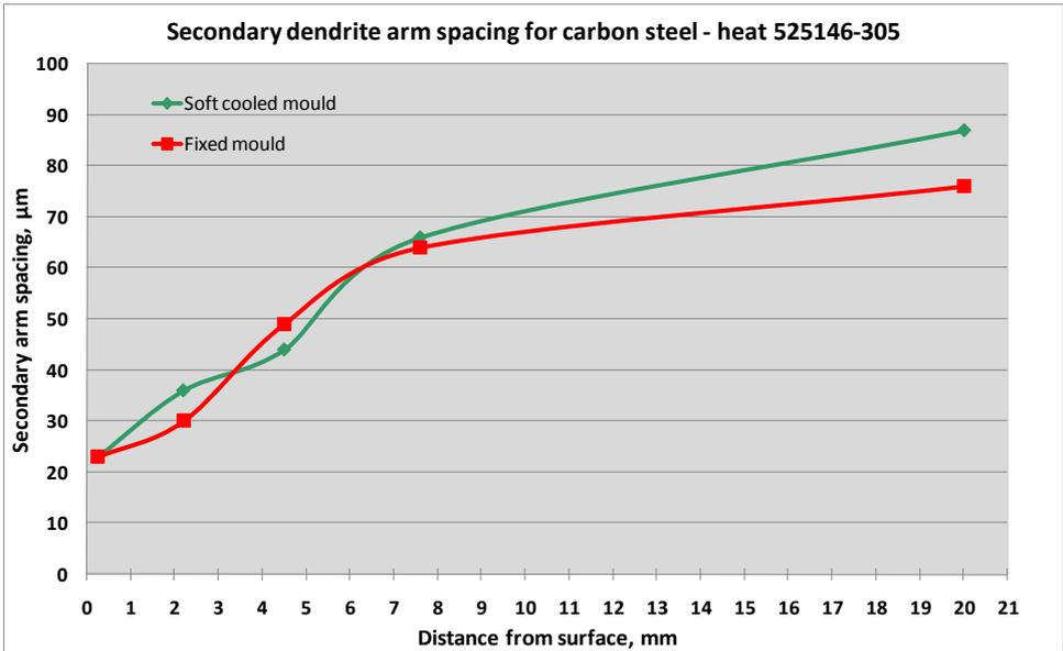
Figure 82. Secondary arm spacing for carbon steel heat 525146-305.
