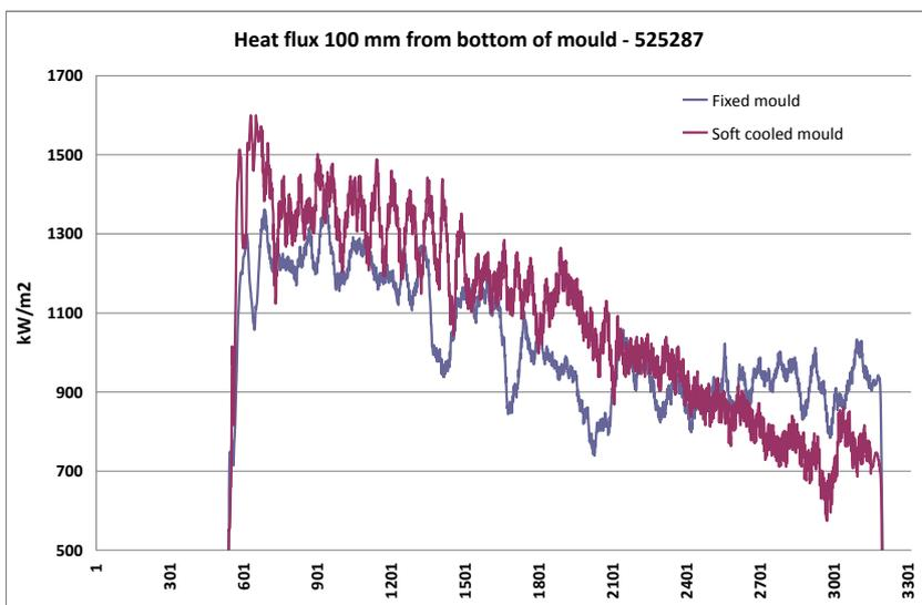
Figure 53. Heat flux at bottom of mould for stainless steel – 525287.
