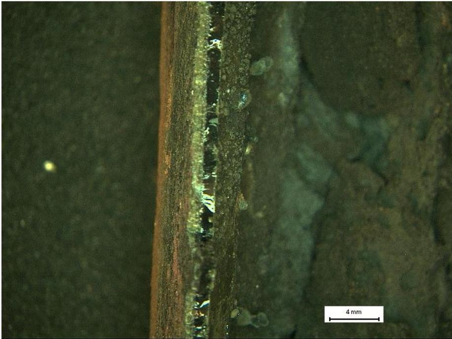
**Figure 35.** Cross section from lower part of the slag rim, partly crystallised from mould surface.
