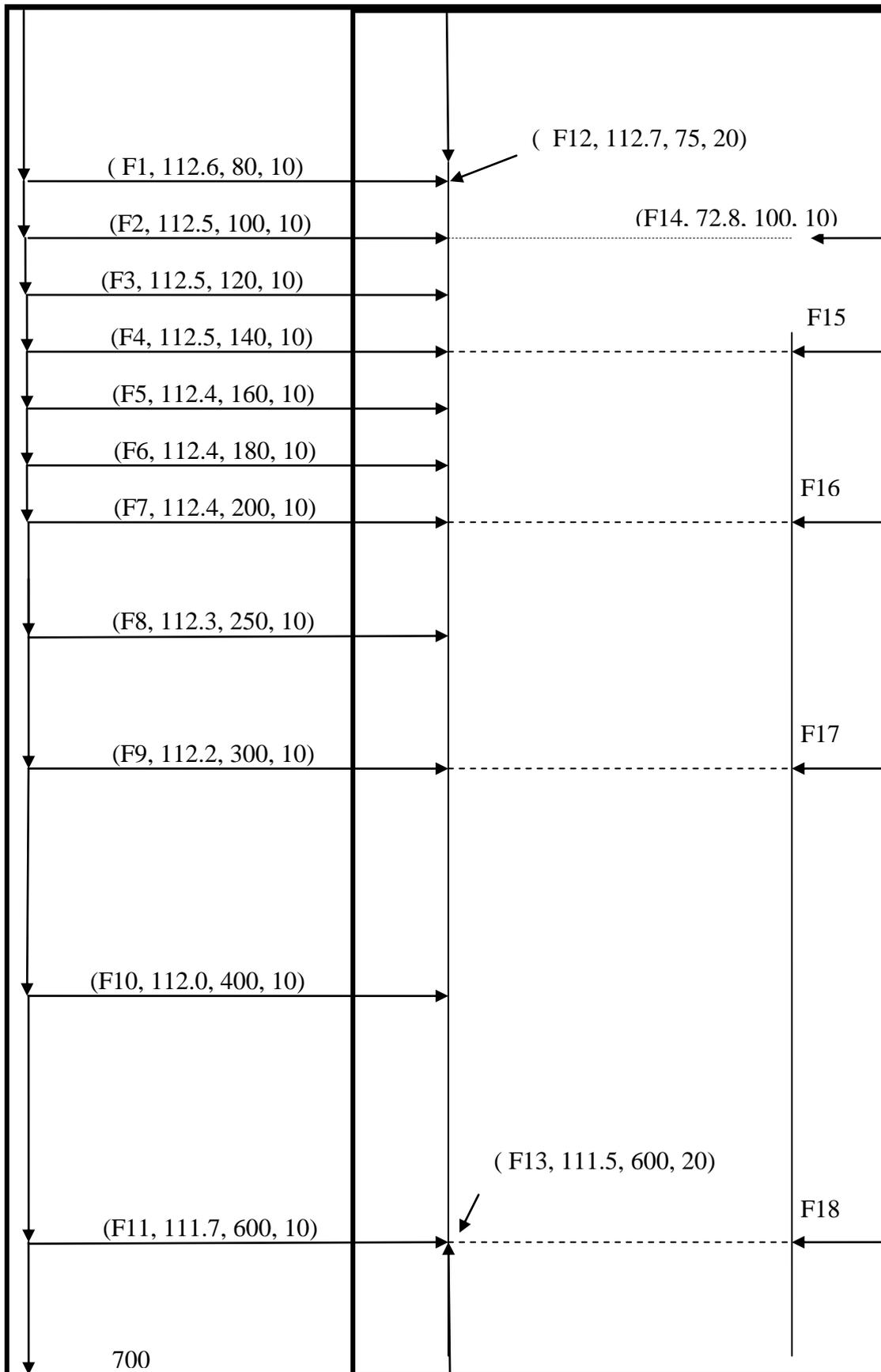
Figure 18. Location of T.C.s for the fixed side.
