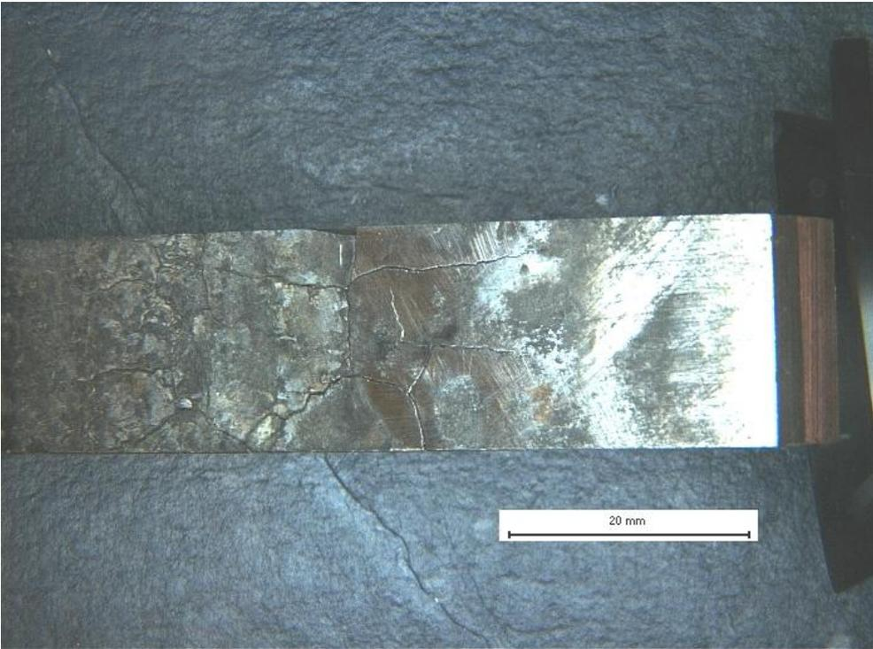
Figure 84. Photo from the surface of the soft cooled mould, 2X.
