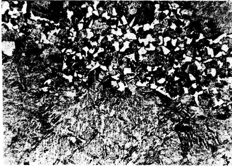
The sabre. Martensite in the blade. Untypical ferrite-perlite structure in the middle part. 500x. Etch. nital.
