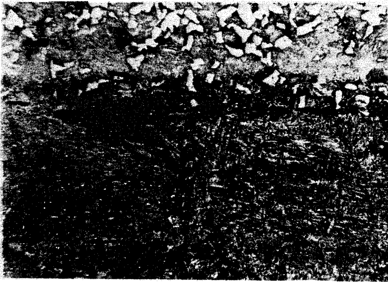
The sword. Microstructure of blade. Large needle of martensite and ferrite - perlite in the core. 500x. Etch. nital.
