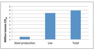
Reduced greenhouse gas emissions on upgrading to high strength steel in the European vehicle fleet.
