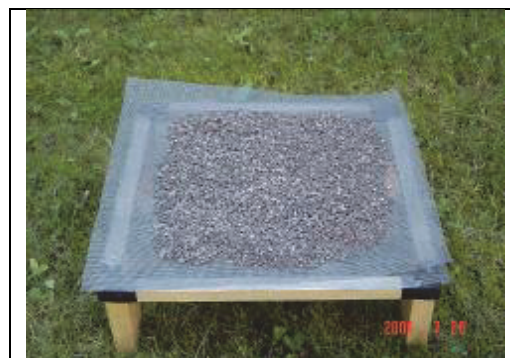
Fig. 2. The experimental setup for ageing of slags in natural environment.
