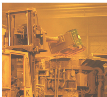
Figure 21 Test of Mo alloying by using FeMoO 4 +C mixtures in 60 ton EAF at Uddeholms AB
