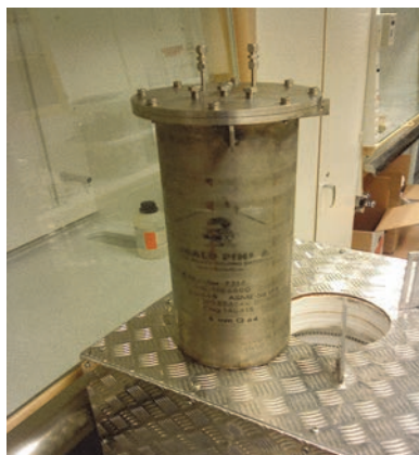
Figure 26 The photo of the big scale unit with slag treatment capacity of 3 kg
