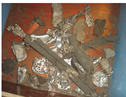
Fig.9. From top to bottom: Al and its alloys, non-metals and ferrous fractions after eddy-current separation (for the size fraction of 32 < P < 50\text{mm} )
