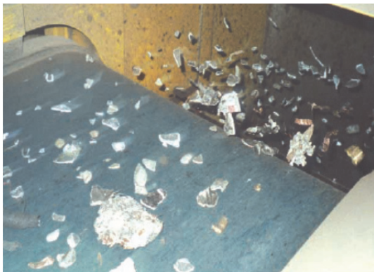
Fig.3. Particle trajectory on eddy-current separator
