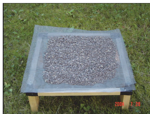
Fig. 1. The experimental setup for ageing of slags in natural environment.
