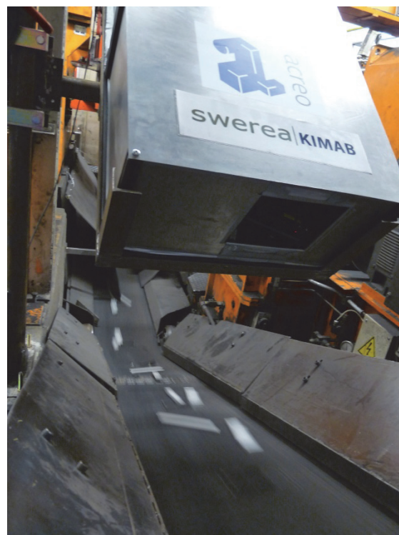
Figure 5. A photograph from field tests at Outokumpu Stainless in Avesta, Sweden. An early version of the LIBS instrument is used to classify internally produced scrap pieces on a conveyor belt.
