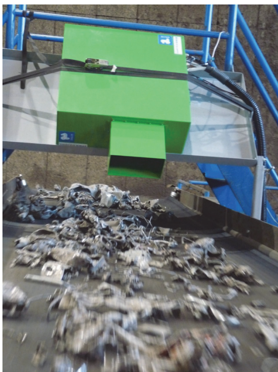
Figure 4. The final LIBS prototype mounted and operating over a conveyor belt transporting shredded scrap at Stena Recycling in 2012.
