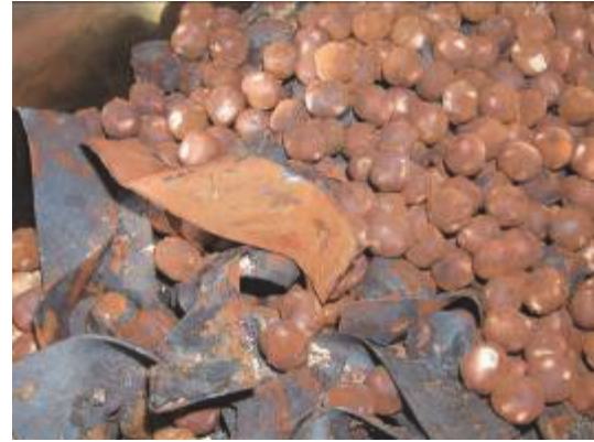
Fig. 6 – Test material from experiment 1. Severe dust formation was observed during the experiment, which can be seen on the white ceramic balls.
