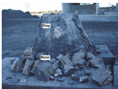
Figure 10 Produced metal and slag from one of the industrial trials using FeSi75.
