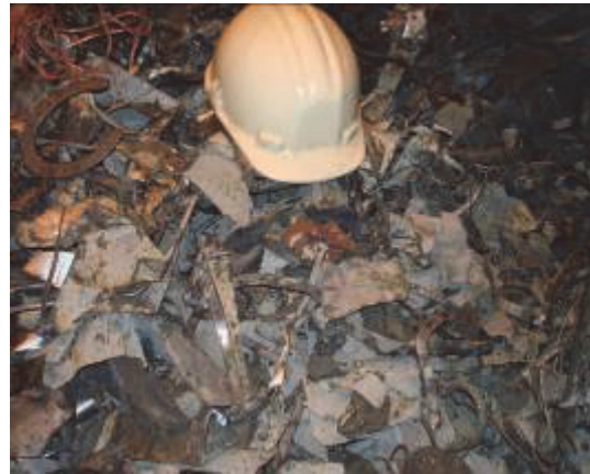
Fig. 4 – Shredded scrap used in the experiment. The picture shows surface-cleaned scrap.
